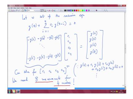
So, with this let us set up the recursive equation right. We can say y of t plus summation I going from 1 to 4 c i y of t minus I equals 0.
