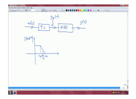
So if you have a discrete time signal here, you up sample this first with a rate l, and then you have this filter H of z that operates on the up sampled signal right, at this stage it is basically Y Y e of n, e standing for expansion. Again it is common sense, because if you have a filter first and then you up sample, you are just putting some zeros, your filtering your doing some operation and then you are up sampling you are inserting 0s in the time domain and what do you want that for right.
