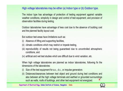
So, the high voltage laboratories which we discussed could be of either indoor type or outdoor type the indoor type facility that is the high voltage which is of indoor type as advantage of protection of test equipment against variable weather conditions. And the design will be simplicity in design and control of test equipment. And there will be provision for observation other facilities during the testing or during the experimentation which is being conducted.
