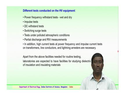
So, as mentioned earlier various type or different test are normally conducted on HV or high voltage equipment include the power frequency at which scientist wet and it has to simulate the rain conditions and dry condition. So, the equipment will be tested for the power frequency withstand could be a 1 minute or a 5 minute time interval wets with
