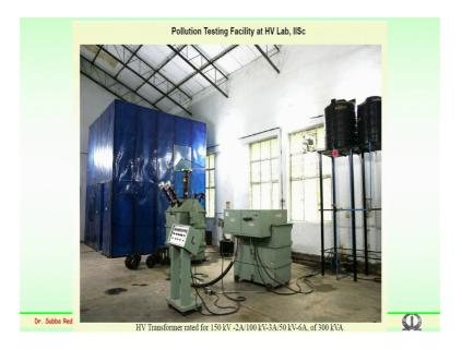
A laboratory has been established keeping this (Refer Time: 26:33) 150 KV 300 KV a source with the 5 meter cube of the pollution or a contamination facility, where insulator strings could be erected inside the chamber. This is from the bushing of the transformer as special high voltage lead is taken inside the chamber consisting of the fog nozzles and the pollution.
