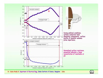
So, we have developed a computer course for the surface charge simulation method particularly looking into the effect of pollution conditions, and the surface conduction field which terminates over the conduction period. So, the profile of the insulator assumes very important prime important this geometry up, in junction this is the cap and this from here to is the creepage or the petticoat region which has been shown here. So, this we have try to carefully counter the pin area.
