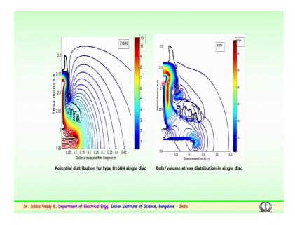
We have also try to simulate the bulk stress the point where the insulator could behalf high stress zone. So, the potential the electric field and the bulk stress have been simulated for various insulators and various strings.
