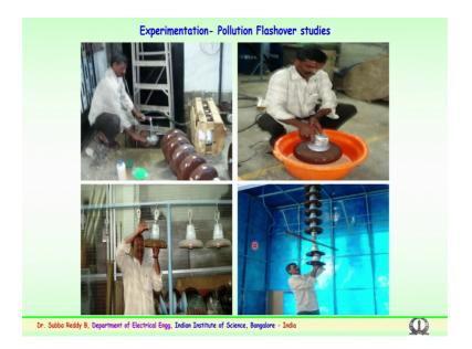
So, the procedure as per international standard is being employed for the ceramic insulator disc and the pollution or a contamination coating is normally carried out, which verification of or the insulator the flashover performance for a normal string and also the strings with the field or reduction electrodes have been carried out and successfully demonstrated for the string consisting of a single disc 2 3 disc in a string.
