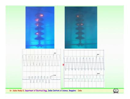
So, lot of experiments I have been carried out for the normal string and the string containing the field or reduction electros which have been developed in the laboratory. We have try to see various configuration for the doubled junction arrangement, a single type of insulators.
