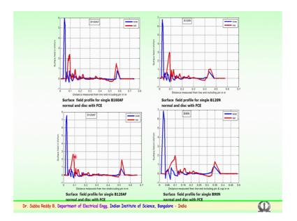
So, we have try to carry out for various type of discs which are being employed in the country. And try to simulate the field control elements and practically used for all the type of insulators.
