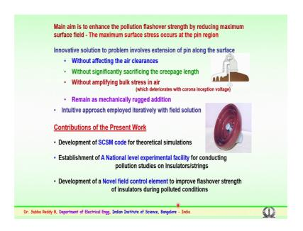
So, effort was made to develop a special field control electros or a field control elements to reduce the surface field. It has been seen that to enhance the pollution of flashover strength is mainly to reduce the maximum surface field.
