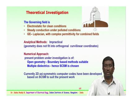
So, we have carried out theoretical investigations, where we have assumed the governing field as a electrostatic particularly for clean conditions; and steady conduction under the contaminated the conditions. So, the theoretical investigations we have used a governing equation as the Laplacian with complex permittivity's particularly for the combined
