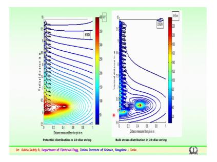
For up to 400 765 KV and all these gives an equi potential plot for a 400 KV transmission tower consisting of 23 disc this shows the bulk stress what is the volume stress which is seen for the insulator string.
