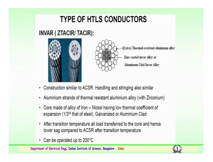
So, we have earlier discussed about the different a types of HTLS conductors we will go slightly go in depth about their construction and also the details of this types of HTLS or high temperature low sag conductors. So, the first one is the invar type of conductors which is a given here this is the invar type of conductors having various thermal resistant aluminum alloy extra conductor which is shown here inside is a zinc coated invar alloy or aluminum clad invar alloy is present.
