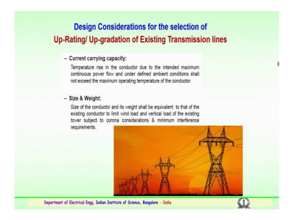
So, there were about the five various types of recently advanced a conductors which are being used for the upgradation or uprating of the existing transmission lines. So, we will discuss about some of the design considerations particularly for the selection and upgradation of the existing lines. So, how the conductors while replacing could be advantages, and what are the necessary consideration design aspect to be followed.
