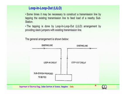
So, before going in for the operating or upgradation of the existing conductors, we will find out some important aspects how it is practically done, and what is the necessity for the requirement for before actually the uprating or upgradation of the conductor is done. So, sometimes it may be necessary to construct a transmission line by tapping the existing transmission line, so which is to feed load say for a nearby sub-station or any other equivalent utility.
