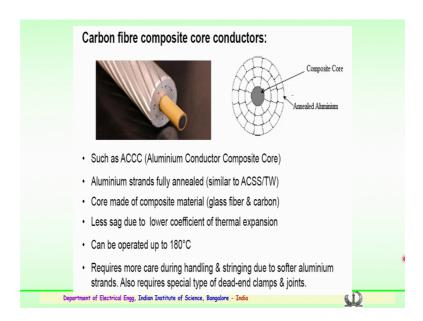
So, fourth is the carbon fibre composite core conductors, this is conductor which is the shown here. You can see number of conductor are arranged in such a fashion with the center being the composite core, all are annealed aluminium conductor. You can see the construction the center being the carbonized core. These conductor sample of the conductor is also shown here.
