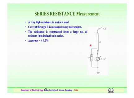
So, series resistance measurement is a simpler arrangement here you can see very high resistance this R is very high resistance is used. So, the current which is flowing through this resistor during the application of the voltage is measured using the micrometer which is a indicator micro ammeter which is used.
