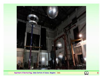
This are this is the damped capacitive impulse AC divider which is being used in our laboratory at the Indian institute of science where for measurement of very high impulse and AC voltages is measured using the divider.
