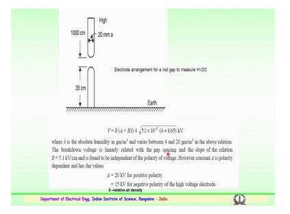
So, this is the typical arrangement as I shown for the rod gap here the voltage could be calculated as delta into A plus BS of 4 in to the square root of 5.1 into 10 to the power of minus 2 into h plus 8.65 kV where h is the absolute humidity in grams per miter cube and this vary between 4 to 20 grams per meter cube.
