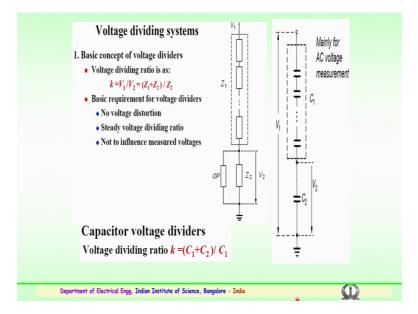
So, the next is the voltage dividers which are generally used after the initial use of sphere gap assembly, the requirements or the further improvements in the measuring aspects for the AC or a DC have been got, and these systems have come into the place where its being used in the laboratories.
