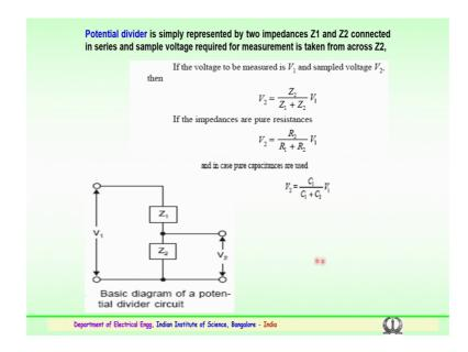
Then simplest divider is the potential divider, and this is the simply represented by two impedances or two resistance is which are shown Z 1 and Z 2 voltage is applied here Z 1 being the very high value Z 2 being the lower value in comparison to the Z 1 that is a resistance could be very low here it is very high.
