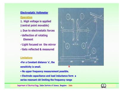
So, this is the typical arrangement of the electrostatic voltmeter which consists of an assembly, consisting of a as mentioned the two arms of the electrostatic plate type of arrangements here. So, you have a indicating scale a small mirror which is here because of the electrostatic forces which we developed this mirror reflects, and this is indicated in the scale this is how the simplest measurement is being done by using electrostatic voltmeter.
