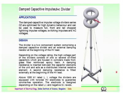
The third type of dividers are known as the damped capacitive it could be impulse or AC dividers. So, it could be used for AC measurement are also for the impulse current and impulse not current impulse voltages or AC applications. So, the application of the damped capacitive impulse voltage dividers are optimized for high dynamic behaviour
