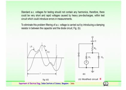
So, for standard AC voltages for testing should not contain any harmonics therefore, there could be very short and rapid raise of voltages which can cause a heavy pre discharges, within the test circuit which could introduce error in the measurement.
