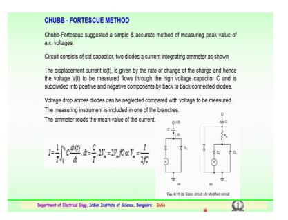
The important and very economical method of measuring the values is Chubb and Fortescue method a famous method; chubb and fortescue suggested a simple and most accurate higher accurate method for measuring peak value of AC voltages, this is in comparison to the sphere gap and other methods this is much more accurate.
