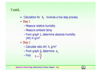
Further, calculation for K 2 is very important this involves two steps that is two step process for calculation of K 2. The step one is to measure the relative humidity. How to do that, we will discuss about it. So, first step consists of measuring the relative humidity then measure the ambient temperature of the experimentation performed.
