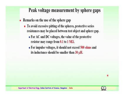
So, peak voltages are measurement was a concept which was initially being used and even till date for the calibration and measurements sphere gaps are also being used in the laboratories high voltage laboratories and the texting laboratories. Few observations on the use of sphere gap, it is advisable to see that excessive pitting on the spheres have to be avoided. During the break down, continuous break down there could be pitting near
