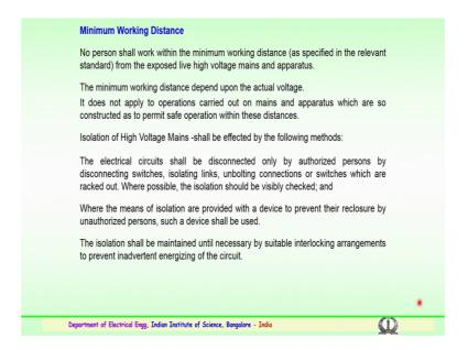
So, these are the hazards which could be effected by the radiological or the field effects, in substations very important hazards. So, what do the precautions have to be taken by the personal working in the substation or in the electrical utilities?
