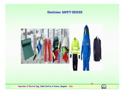
So, these are some of the various safety devices, which are used by the utility personal or the electrical staff or technicians in the substations. This could be of insulating mats it could be insulating gauntlets or a gloves suitable helmets, which are to be used and the insulating dress which is very important for the live line maintenance personal.
