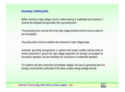
So, finally, is the grounding or the earthing stick which is very important device, where before touching high voltage circuit or before living it unattended and exposed, it must be de energized and grounded with a grounding stick or earthing stick. So, this grounding stick must be left on the high voltage terminal permanently connected until the circuit is about to be reenergized in case of maintenance.
