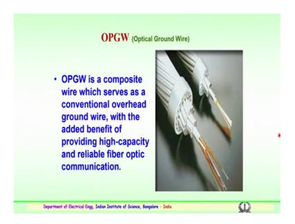
So, the optical ground wire or OPGW as it is a shown here, is basically a cable here you can see the cable here. It is similar to the ground conductor and the size of the cables
