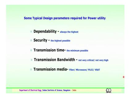
So, some typical design parameters which could be required for the power utility engineers, he is the important being the dependability. This has always the highest requirement. So, the dependability followed by the security have the highest possible dependability.
