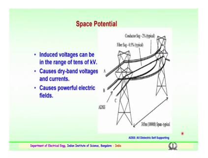
So, this is a example of how between the two towers the conductors which are connected, one example is all dielectric self supporting cable that is the optical cable, which is being connected for communication purpose. You can see here in case a typically the conductor sags between two to five percent. So, during that period there is a
