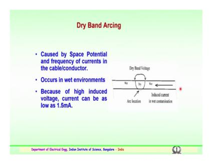
There the dry band arching is again caused by the space potential has mentioned. And here the frequency of the currents in the cable or conductor and depends upon the type of potential the magnitude of the potential, and how much is a induced current during the wet or the moist conditions. So, because of the dry and wet band which are formed on the surface and because of the induced currents there could be a small arching which are known as a dry band arching.
