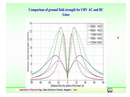
So, similarly comparison for the ground field strength, for both a ultra high voltage AC and DC transmission lines was estimated, and a comparison is made here. You can very clearly see the comparison conducted for both ultra high voltage AC and DC lines, for the electric field strength this y axis shows the electric field strength verses the distance a from the center of the tower.
