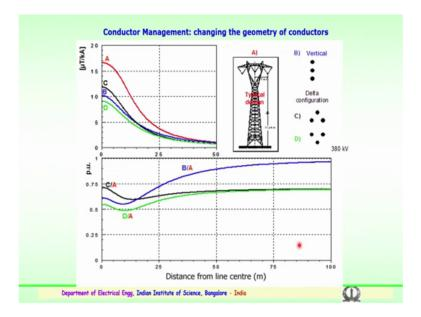
The second point the one was the clearances a height, the as mentioned earlier the conductor management a very important, this we have also seen that is a conductor going in for the different configuration. And also the conductors being going in for a transposition this will help in the reduction of files fields electric fields.
