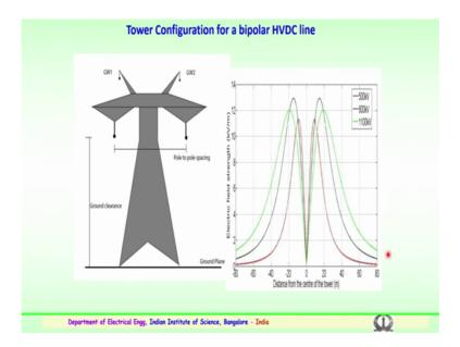
This is a similar study conducted for the tower configuration for a bipolar HDVC transmission lines for a various voltage levels, a 500 kV 800 and 1000 kV lines from the data which is being obtained in the literature for the tower details have been the data for the tower details have been obtained from the utility and also from the literature.
