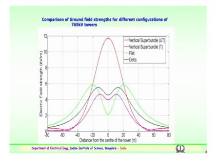
Again comparing for the ground field strengths electric field strengths, for different configuration again for the 765 towers, you can see that for various towers we have carried out the simulations. This simulations results very clearly show that for the different towers and also for the transposition and a untransposed ah, conditions that is a vertical super bundle type untranposed and vertical tower with a transport system, and also for a flat tower and a delta type of configuration.
