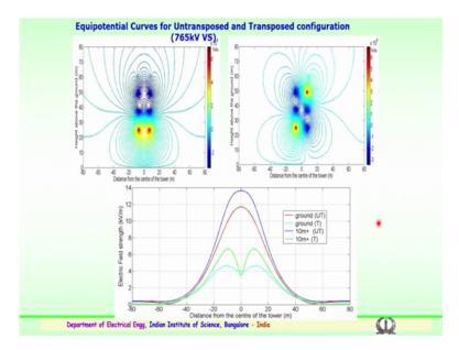
So, is there some of the things we some of the magnetic field and electric field values which have been simulated in the using developed software. So, for a 765 kV the curves have been shown both for the untransposed, this is for the untransposed normal tower 765 and this is for the transposed tower you can see height above the ground verses the distance from the center of the tower.
