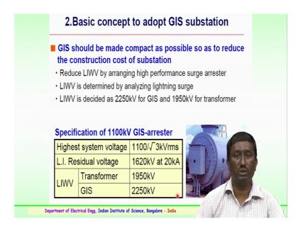
And going in for this; so, to reduce the lightning impulse withstand voltage, a lightning impulse withstand voltage by arranging high performance surge arrester could be done and also is determined by analyzing the lightning surge. So, this can be again considered to reduce the cost. So, lightning impulse withstand voltage is decided as a 2250 for gas insulated substation and 1950kV for transformer for a particular voltage level of mentioned shown here in the table.
