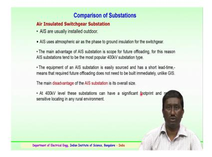
So, we will compare various substations importance comparison of air insulated switchgear substation. So, generally air insulated substation are installed outdoor that we have discussed. So, air insulated substation uses atmospheric air as the phase to ground insulation, so air is basically used as an insulation; that is the clearance from the metal to the ground is being maintained with the insulating media being the surrounding air of for any switchgear.
