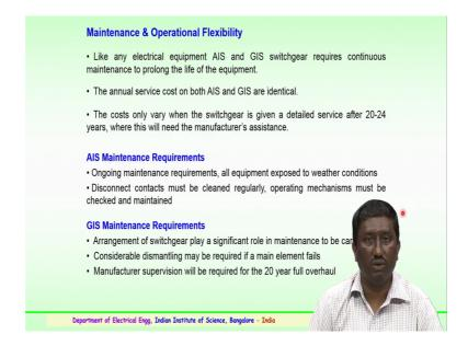
About the maintenance and operational flexibilities very important point, so like any electrical equipment; it could be air insulated or a gas insulated switchgear. These require continuous maintenance very important because the maintenance done normally to prolong life of the equipment or the insulation of the equipment so that it last for a last period of time in the service.
