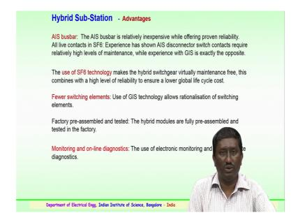
So, what are the advantages of going in for this hybrid substation, so hybrid substations you have the air insulated substation busbar that is the busbar is relatively inexpensive while offering proven reliability which has been used for the long period of time. All live contacts in sulfur hexafluoride; that is SF6; experience as shown that air insulated substation.
