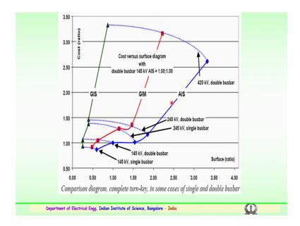
This generally this graph as you can see it shows, a general comparison diagram for three technologies; gas insulated, air insulated and the hybrid insulated or a going in for that hybrid substation. This shows the cost ratio in the Y axis and the surface ratio; for various busbar, the comparison made for 145 to 245 and a 400kV busbar with single and double bus.
