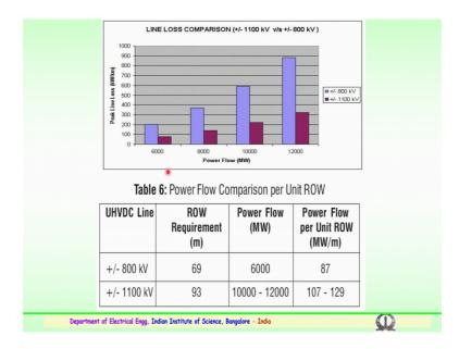
This gives a line losses comparison for both 800 kV and 1100 kV DC, you can very clearly see for transmission of 6000 megawatts; comparison between 800 and 1100 HVDC lines, very clearly this is the peak line losses which you see kilo watt per kilo meter is a Y axis and X axis being powerful in mega watts.
