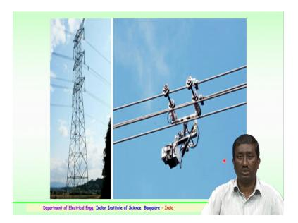
So, this will be very helpful one such robot is again shown here for the very high a transmission aspects; which has been recently developed and which is very very useful for the transmission utility engineers to rectify the conductors, the spacing arrangements in mechanical damages happened to the conductor of the spacers or to any other hardware component on the transmission towers.
