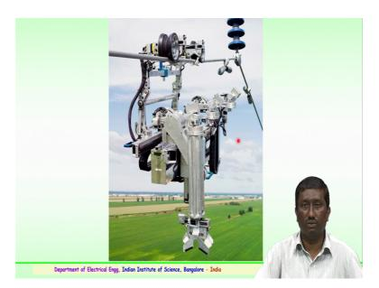
So, this is how the robot is being used to see and check the starters of the conductor, the healthiness of the conductor and the information is been given to the utility engineers
