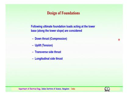
How the design of foundations? Again considering various aspects following ultimate foundation loads which acts on the tower; at the tower base, along the tower slope are
