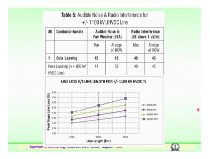
So, similarly audible noise and radio interference limits have been also estimated for 1100 kV. Here again comparing with 8 conductor Lapwing type of conductor arrangement which is 38.05 dimension; you see that audible noise, the maximum estimated should not be increase 45 decibels and at the edge of the right of way, it should not increase more than 43 is a estimated value and going in for hexa; that is a 6 a bundle Lapwing presently which is being used for a 800 kV, the value is 41 and 39.
