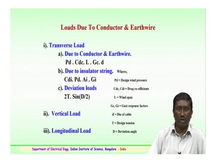
And the loads due to conductor earth wire and insulator strings have also to be considered. Again this type of loads whether the loads are towards the transfers load or it is due to the conductor and earth wire or due to the insulator string or due to the deviation of the loads because of the wind at that area, what type of vertical loads or it is loads because of longitudinal compression tension.
