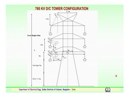
So, this gives the line diagram of the tower configuration of 765kV DC tower which is been used. So, you can see the total height and the maximum sag which would be and the minimum clearances and number of conductors which are employed the hexagonal type of arrangement you can see and what is a minimum clearances from the ground to the phase metal part; that is a tower edge minimum of 4.5 and the ground to ground is 23.5 meters.
