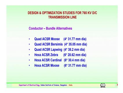
And conductors bundle alternatives, which were employed for the double circuit again the data was from the previous single circuit lines and here the adoption for double circuit was they have adopted quadruple that is a 4 conductor ACSR; all aluminum steal reinforce, the moose conductor. The moose is 31.77 is a diameter of the conductor 4 being; 4 conductors of 31.77 dia were used, when the moose were employed.
