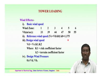
So, how to consider the tower loadings very important aspects we have discussed about the conductor mechanical loads, insulator strings, the wind effects, some of the zones where the transmission towers are been constructed. So, these wind effects for the tower loading have to be considered before the estimating the actual tower loading apart from the insulators, the line conductors, several accessories, wind aspects.
