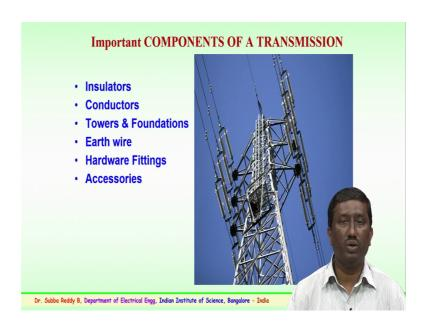
So, this shows the most important components of a transmission as network transmission system. Example is shown here a transmission tower, where the tower consist of are the following components which are very important. Insulators the first is the insulator.
