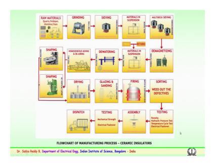
A very quick look into the flow chart of the manufacturing process, for both the ceramic and the polymer will show you how much difficulty is to manufacturer porcelain or a ceramic insulator on the time period which takes place for the manufacture of the ceramic or a porcelain insulator.
