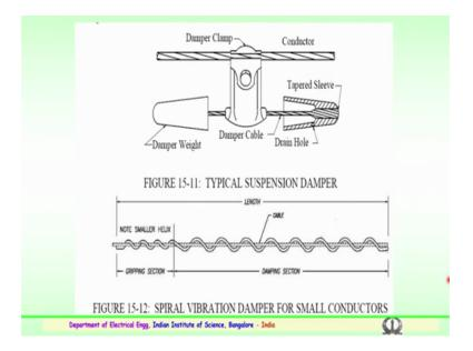
This is again a typical suspension type of a damper the conductor is here, the conductor the damper is made to fix on the conductor intentionally drain hole and a damper weight on both sides. And this sizes are a slightly different, they are not in equal weight. This is mainly to reduce the frequencies and to curtain the frequencies of four different frequencies with the conductor sees. So, this helps the proper containing the frequencies form due to the Aeolian and other vibrations.
