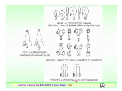
So, these are various types of the connectors a hook which are being used for the transmission system, various type of a hooks for the insulator conductor and the accessories which are being employed for the transmission and also for the distribution systems various types or different voltage levels.
