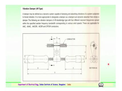
So, vibration damper important component that was of spacer damper. This is a vibration damper are there are different types. So, one is the 4R type of arrangement what is known as. A damper is normally defined as a dynamic system capable of damping and observing the vibrations, which are conductor sees in a transmission system and subjected to a forced vibration. So, it is more appropriate to designate a damper. As a damper come dynamic absorber then simply a damper that is very important.
