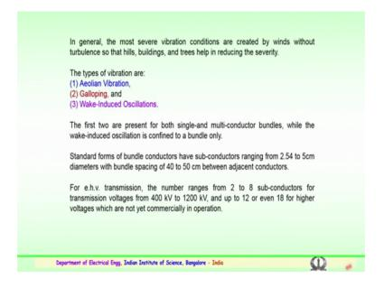
So, in general most severe vibrational conditions are created by winds without turbulence so that hills - a mountainous areas, buildings and trees particularly help in reducing the severity. So, any turbulent winds could be blocked by these high rise buildings, hills, trees an extent, but the type of vibration some other types of vibration or known as the
