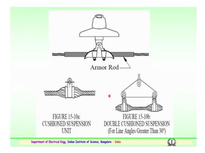
This is the armor rods which initially will suppress the oscillations you can see from the insulator string after the necessary clamps. The twisted conductor is armor type of conductors which either side of 5 meters on the conductor are twisted to see that the vibrations caused by Aeolian or galloping or wake-induced oscillations are reduced in case of a single conductor bundle.
