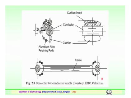
So, this is one of the type of spacer. The spacer for two-conductor bundle you have one conductor other conductor the distance between the spacer that is the aluminum metal
