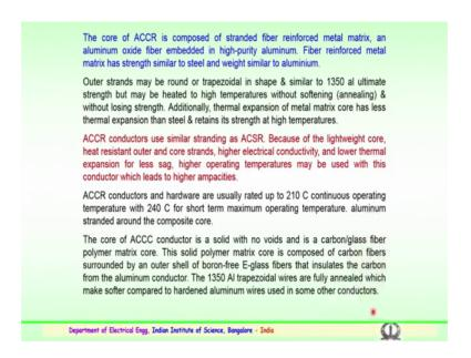
The core of this high temperature high current conductors for ACCR is composed of strands with fiber reinforced metal matrix is an aluminum oxide fiber embedded in high purity aluminum it has to be noted here the fiber reinforced metal matrix are strength a similar to the steel and weight similar to the aluminum.
