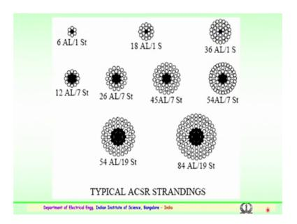
Apart from this zinc based coatings, these are the typical aluminum conductor steel reinforcement standings you can see here 6AL slash 1 t, this represents the center conductor is a single conductor, one conductor of steel surrounded by 6 strands of aluminum. So, 6AL is 6 strands of aluminum the center conductor is one of steel. So, this is the nomenclature similarly it could have a one steel center conductor and 18 aluminum which are standard as shown here.
