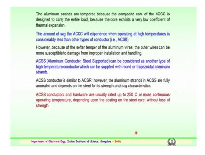
Here the aluminum strands are tempered because the composite core of the high temperature conductors or ACC conductor is designed to carry the entire load because the core exhibits a very low coefficient of thermal expansion.
