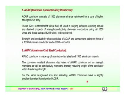
The fifth is the ACAR aluminum conductor alloy reinforced this consist of again 1350 aluminum strands reinforced by a core of higher strength 6201 alloy. So, this 6210 reinforcement wires may be used in varying amounts allowing almost any desired property of strength or conductivity that is between conductors using all 1350 conducting
