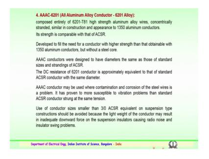
Before these triple AC 6201 that is the all aluminum alloy conductor 6201 is alloy of aluminum this is composed entirely of a 6201 T81 alloy with the high aluminum strength where wires concentrically stranded similar in construction and appearance to the previous 1350 aluminum conductors and it is strength is comparable with that of the aluminum conductors steel reinforced first conductor.
