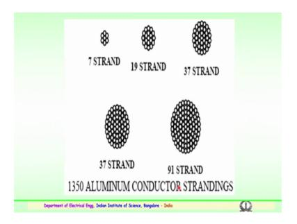
Typically aluminum conductor that is strandings are of this measure we have a 7 strand we have 19 37 strand, 37 91 strand. So, 1350 aluminum conductors strands of typically in this type.
