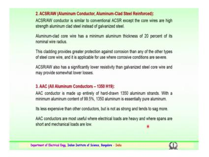
Aluminum conductor aluminum clad steel reinforcement. So, here ACSR AW conductor is similar to the conventional earlier ACSR conductor except the core wires are high strength aluminum clad steel instead of galvanized steel.
