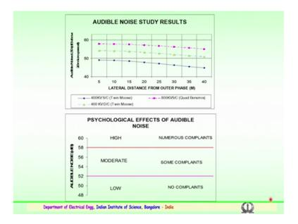
So, similarly audible noise a lot of studies have been carried out for 400 that is a EHV and ultra high voltage lines. And you can see the audible noise in decibels versus the lateral distance from the outer phase conductor phase towards the ground side. It is very clearly as that from the tower if you move away towards the distance in case of 400 kV single circuit twin moose you can see somewhere from 48 decibels it reduces to a lower level.
