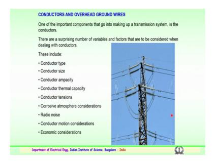
So, conductors and overhead ground wires you can see various conductors are from insulator string various types of conductors are used for transmission. This is the overhead earth wire or a ground wire which is connected to the top most point of the tower to tower. So, this in case of lightning protects the entire tower the conductors are the insulators. So, that the lightning strikes and it is grounded. So, this earth wire or ground wire helps in taking the search to the earth or a ground.
