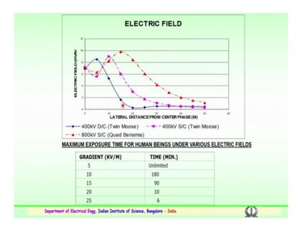
The graph gives the electric field kilo volt per kilo volt versus. Here the lateral distances from the center kilo volt per meter for lateral distance from the center phase in case in meters very clearly shows 3 different curves here. So, one the black curve corresponds to the 400 kV double a circuit employing a twin moose conductors that is a 2 conductors of moose make that is a 2 moose conductors are used in a double circuit.
