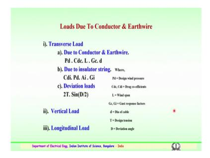
So, how the loads particularly due to the conductor and the earth wire which are connected to the tower are calculated. So, these are important considerations. The loads due to transverse load have to be bear in mind. This is because of the conductor and the earth wire. So, a simple formulae is being used for the calculations the details are for the transfer transverse load due to the conductor and earth wire it is Pd Cdc L Gc and d these are for 5 factors to be bear in mind.
