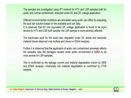
For the high temperature vulcanized and liquid silicone rubber samples, both for the acidic and normal contaminants are analyzed, both under AC and DC voltage applications. Under different environmental conditions were simulated using the acid rain affect which is available the details available in the literature as per the data
