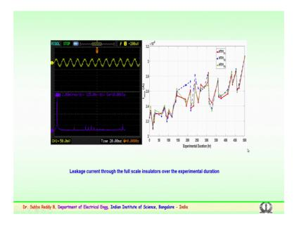
So, experiments have been perform this is a typical leakage current wave form which shows here has been for a particular one sample, this shows the ah the frequency component involved in that at that junction which is form through the which is got from the oscilloscope, the over the period of time this typically gives the experimental duration for 500 hours.
