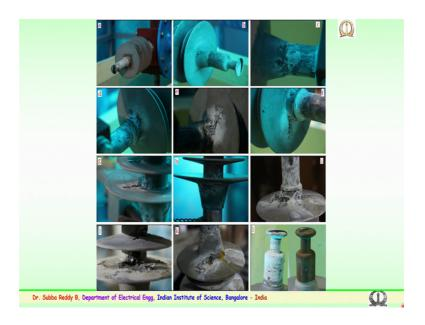
So, further to that not only the surface degradation, some of the places a puncture science have been noticed and the pin or a metal corrosion has happened on many of the samples, and in particularly in acidic treated samples a more degradation more surface rupture and the pin getting corroded have been visible much more in compared to the normal contaminant. So, several of the experimentations have been conducted and evaluated for various types of samples.
