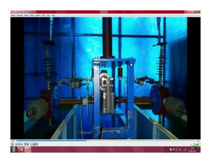
So, this cycle of rotation and the oldest stress which is being seen will be continuously applied for 1000 hours, and the experimentation is being ah conducted and during the experimentation the flow of leakage current on both the sides is measured using the centre box with the protection, employing the digital storage oscilloscope and also national instrument module where you can capture the data for the entire 40 seconds period and during the contact of high voltage.
