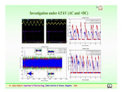
So, this is how the performance particularly for the inclined plane arrangement has been done. During the process, the leakage current and the various samples this one of the experimentation is conducted for 4.5 kilo volts; both for AC and DC application. You can see the discharges during the process and this discharges which are of continuous in nature have been again recorded using a national instruments module, where long duration data could be captured and used for analyzing the data.
