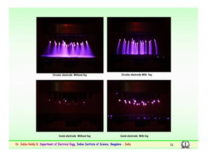
So, during experimentation where normal ambient light; it is very difficult to capture the corona discharges which are being impinged on the sample. So, these could not be taken with the normal photography; the discharges which you are seeing here are being taken with a setting of 30 seconds to capture this. So, the ambient is made completely dark and the photography is taken in such a way with a shutter speed of 30 seconds so that you can capture the discharges.
