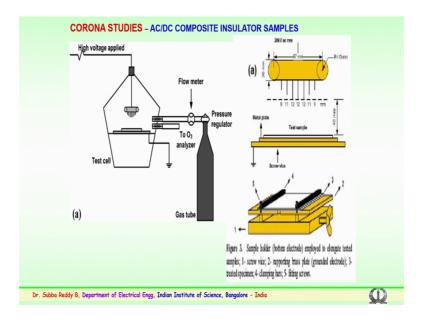
So, corona studies both for AC and DC composite or polymer insulator samples, so it is normally conducted in a experimental arrangement; test cell, where intentionally with a use of a corona needles; the corona various types of a needles could be used either a circular type of needles where of uniform in nature or non uniform type of needles like which looks like a comb type of electrodes.
