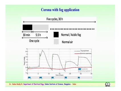
So, how the cycle is being designed that is application of voltage, application of fog could be of normal fog, a mist or an acidic fog which comprises acidic components; which simulates the acid rain. So, this methodology is being adopted; where depending upon the number of hour, say the cycles which is being presently shown is for 30 hours period example, the experiments have been conducted up to 100 hours also. So, for example; if it is a 30 hours; initially 6 hours is considered as one cycle.
