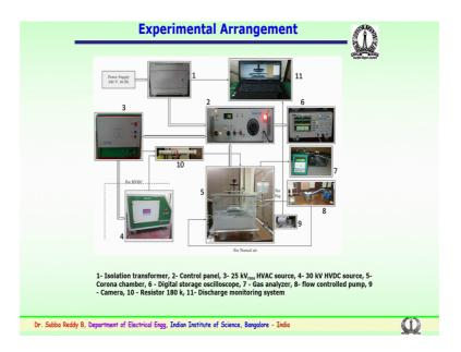
So, experimental arrangement with normally corona experimental arrangement consists of the following. So, we have a corona important is a corona control chamber here; we have a supply, power supply; a control panel we have high voltage AC, high voltage DC. So, for studying of AC voltages or studying the DC voltages both the AC, DC generators are here with a resister to limit the current in case of the flashover happens across the insulator sample here.
