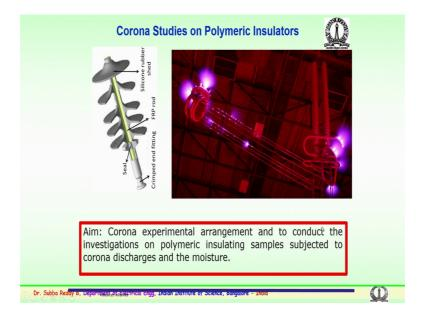
So, the first we would like to look focus on the corona aspects: the corona studies on coronal insulators. So, as mentioned earlier just for information; we have a polymer insulator which mainly comprises of the crimped end fittings, both the side the end fittings are there. Apart from that, we have a fiber glass or rod f r p rod; from the metal to metal and we have silicon rubber or a polymeric sheds which are housed on the silicon rubber insulators.
