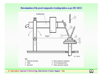
The first one is the determination of the proof of comparative tracking and this stand is as per IEC 60112 standard. Basically, you have on a experimental arrangement which is fabricated; here you have two electrodes that is where the electrodes are of platinum edges with a brass electrode arrangement. Then, you have the weight to see the proper mechanical force which is kept on the sample; this is the sample. The fifth which shows
