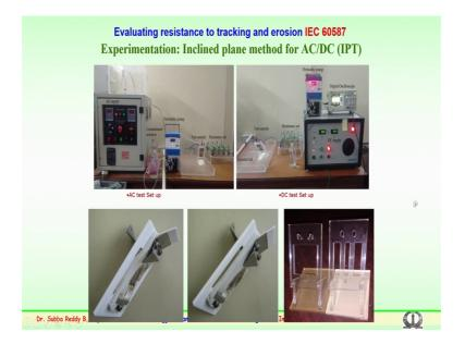
So, this shows the laboratory evaluating resistance to tracking as per the 60587, which also knows the inclined plane arrangement. So, we have tried to make both for AC and DC, so DC; this shows the arrangements for the AC experimentation. The second one this shows the arrangement for DC arrangement, so DC the standard has not been evolved.
