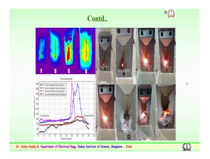
So, this is how the performance is monitored and this gives the experimental performance for various types of samples. You can see the surface rupture or surface erosion which is happening on the samples at different locations, this is a ground electrode; you can see over a period of time because of the continuous the flow of contaminant the surface the electric stress the discharges happen in how the erosion happens near the surface; near the ground end.
