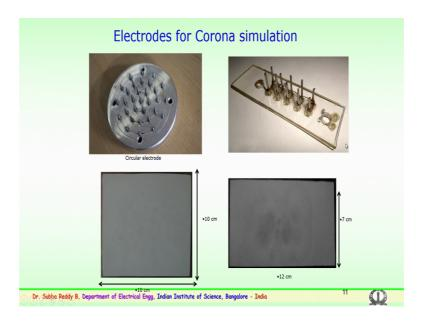
So, some of the methods which are being employed in the lab; so, we have tried to make two types of electrodes. So, one is particularly the uniform type of electrode consisting of 33 needles to simulate the uniform corona. We have other type of electrode which is shown here, this is again non-uniform type of arrangement to create a non-uniform corona, it is not a uniform needles are not employed here. So, we try to come simulate
