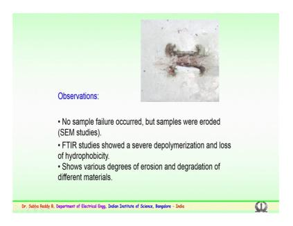
So, this is how some of the observations where between the electrodes; the sample, there is a erosion which has been observed so, but no sample failure occur during the process. All the samples were observed to be eroded and when the scanning electron microscopy studies were carried out and the studies from the Fourier transform; infrared study showed that a severe depolymerization and loss of hydrophobicity; particularly the water repellent activity of the rubber had lost the property.
