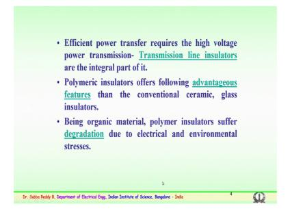
So, you know that for efficient power transmission require the high voltage and transmission insulators are which found the integral part are very important components either it is a ceramic glass or a polymer. So, polymer insulator offers many advantages then the conventional ceramic or a glass. So, being organic they suffer degradation this is a very important point to be noted, this is due to electrical and also environmental stresses.
