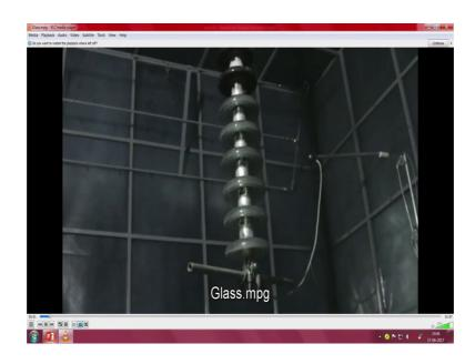
So, one such example you can see here, this is the chamber especially made for pollution studies where you can see the having glass insulators in 6 insulator are in service.
