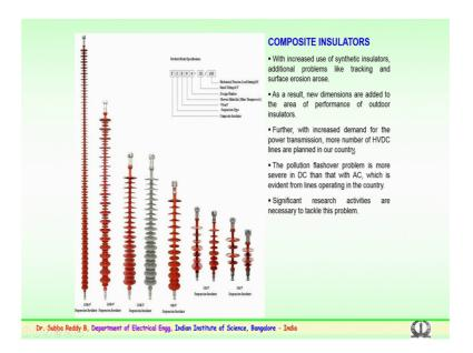
So, the composite insulators increased over the period particular in the country; for a decade also we are being using it for distribution voltage levels to the ultra high voltage a levels both for AC and DC applications; with increased use of synthetic or a composite type of insulators the utilities are facing additional problems particularly like tracking and surface erosion.
