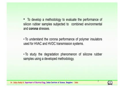
So, for these to carry out the facility it is necessary to develop a methodology how to evaluate that is very important to check the performance of these composite insulators when subjected to combined environmental and also corona stresses. So, this is very important point to be noted.
