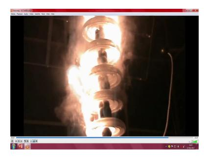
So, this is one of the experimentation for conducting the wet on pollution; this you see the entire flash over across the shrink during the flash over you are also observe the fumes of hot fumes which are like a smoke coming out of the during the flash over process.
