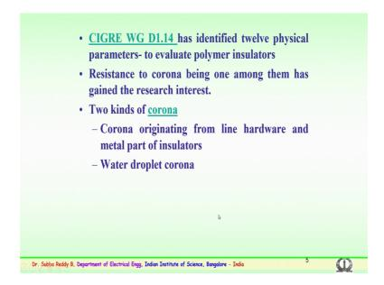
So, CIGRE working group which I mentioned earlier, which is an international body or a council for large high voltage systems working group D1 14 has mentioned as identified 12 physical parameters to evaluate polymer insulator. So, resistance to corona is one among the important which has gained the research interest. So, many people are a focused towards this subject and are being working towards the remedial or trying to see how improve mental aspect could be done.
