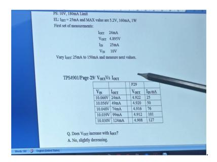
So, the big summary here is that V out is quite stable for whatever output load currents which are changing, the input the output voltage seems to be stable. Of course, if the output current requires 24 milli amperes it has to come from the power source and the that power source induced was the power supply the input current has to increase and therefore, you can see that the input current is the power supply is able to provide that input current.
