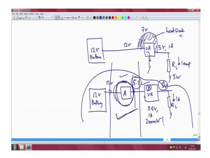
Perhaps you have a one volt battery you are interested in generating 5 volts and the output, and essentially you are going to give an input of 12 volts, you are generating an output of 5 volts. And output which means and let us say the current requirement is 1 amp for the load one amp is flowing through this.
