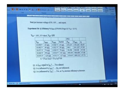
So, now what we do is we change the input from 8 to 10 volts and we again you know vary the output load current using that electronic load from 24 to 124 milliamperes you find the efficiency has dropped right. Now you can answer this questions is IOT equal to I in yes almost is efficiency influenced by I output the load current no not influenced is efficiency a influenced by input yes as V in increases the efficiency decreases. So, this is the big summary stop.
