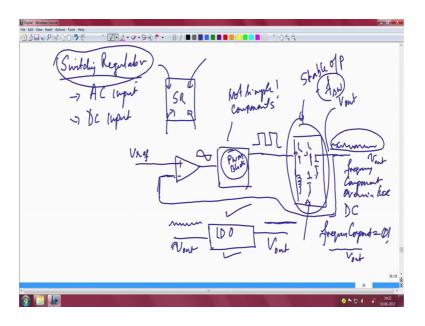
It is a switching regulator because if it is switching it can take AC input it can also take DC input.
