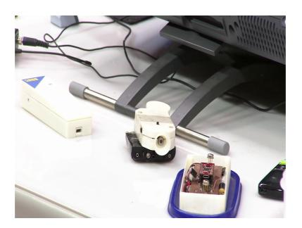
You have this nice little sensor here, that sensor that you see those are inside here this is a battery pack we did this in the lab. So, I just put a lab scale battery pack and what you see inside is essentially a medical grade it is basically a medical grade IR thermometer, medical grade thermometer.
