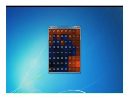
These 64 grid eye pixel elements that you see are essentially indicating the temperature, if I change the direction of the grid eye sensor this will also change. You can see let us first focus this grid eye sensor on one particular in one particular direction. So, let us now refocus back on this grid eye sensor. So, let me put the grid eye sensor like this, now
