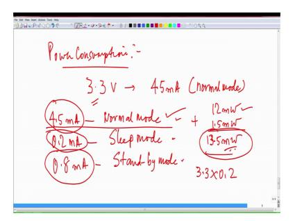
First thing you would be worried about is what is the power consumption of such a sensor; well what we have done is we have operated this at 3.3 volts and it takes a current typical current consumption of this sensor is in let us say 4 is actually 4.5 milliamps under normal mode. There are other modes that the sensor supports which
