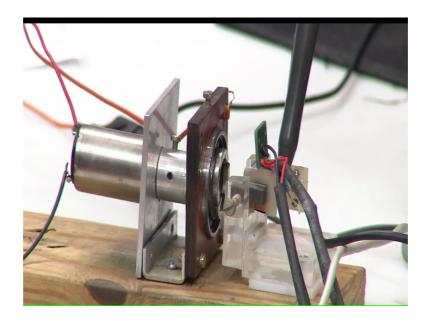
This you see is a coil, this is a coil this is essentially a coil and it is actually inducing certain electricity certain amount of energy because of these neodymium magnets which are attached for the purposes of sensing the temperature of the bearings.
