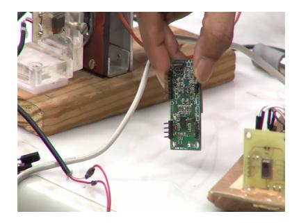
We mentioned about a board which was like this, you can see that this is the p c b that we developed in the lab essentially has interfaces for connecting these wires directly to this system and has a sort of an energy storage device which is here this is a super capacitor or an ultra capacitor as they are called which essentially stores energy for measurement of this bearing temperature.
