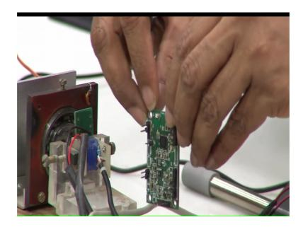
Rectify the supply and store that energy on this capacitor here this is a super capacitor, and use this energy for the purposes of powering the hall sensor for temperature measurement.
