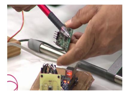
So, you see this little white portion here this is this white portion here essentially is the chip antenna of a Bluetooth low energy module, which is integrated into this SOC. This SOC is essentially a system on chip as it is called is from the; from a company called Nordic semiconductor.
