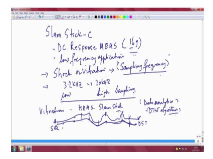
What it these slam sticks that we have it is called slam stick slam stick-c and this is essentially a DC response MEMS equipment, shock and, and vibration is that you must be careful about the sampling frequency. If you do not sample that enough at a higher at the a the required frequency you will end up losing, because if you are points are very spars then you may actually end up losing the required, you may end up losing the catching the right g value.
