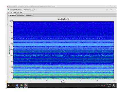
So, spectrogram essentially we will tell you, this is for the x axis, this is for the y axis and this is for the z axis, they are the this spectrogram essentially we will tell you how the frequency and the amplitude changes with time of course, essentially it is another way of representing the, so essentially it is after doing and FFT. So, how it basically where is you can see that, how this particular frequency where is over time.
