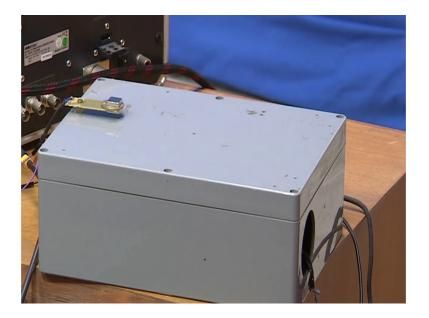
What I so show you here, is this platform is actually now switched on as you have seen Abhishek just switched it on. It is vibrating. This is the vibration energy harvester. It is basically not bounded, but it has a tipping mass here we can see, there is a tipping mass that has been applied. And it is fixed to this surface which is vibrating using this screw and we are trying to see what actually happens in terms of the output voltage.
