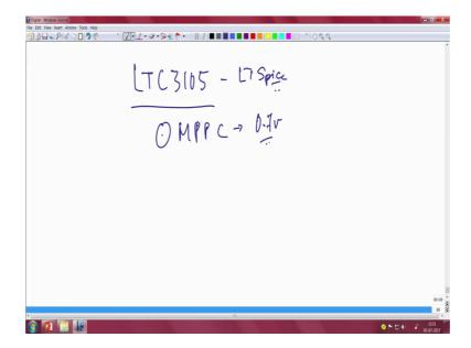
It is feature of using OMPPC, where you are setting this maximum power point control feature. If you have let us say two panels which are stacked in series, you may actually want to set it to 0.7 volts and ensure that the panel never collapses and yet you are able to extract energy power from the panel and store it into maybe a capacitor or trickle charge into a battery, ok.
