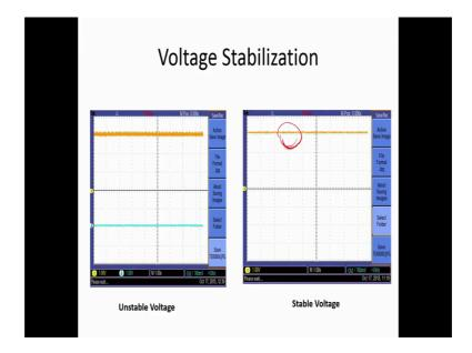
So, you could build that. The system is very stable when we were actually making a measurement. You can see that the voltage that developed across the microcontroller in the first picture that you see on the left side here, actually was quite a lot of voltage was really unstable and we had to do lot of nice tweaks in order to get back a nice good way form here which will allow us to use and power the pulse sensor effectively.
