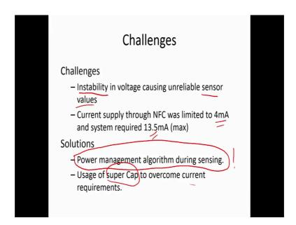
So, that correction was required. So, challenges were there was instability in the voltage causing unreliable sensor values. Current supply through the NFC was limited to 4
