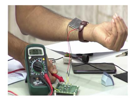
For this let me show you demonstration of another kind of device which essentially is called the thermoelectric generator. So, you can see this is TEG. What I have here is a Thermoelectric Generator and there is obviously it is not very thick. There is a hot side and then, there is a cold side and I will show you. So, what I have done is, I have connected it to a PCB which is right here.
