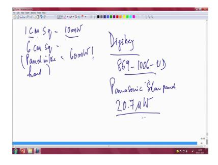
1 square centimeter should give you 10 milliwatt. This is actually 6 centimeter square. In the hand panel in the hand I have just put it here. This should give you 60 milliwatt of power. So, on paper it appears that this should give you 60 milliwatts of power, but I just looked at the manufacturer's specification. This is available in Digi-Key. You can bite from Digi-Key and it has a part number. I can give you 8691006 and this is from
