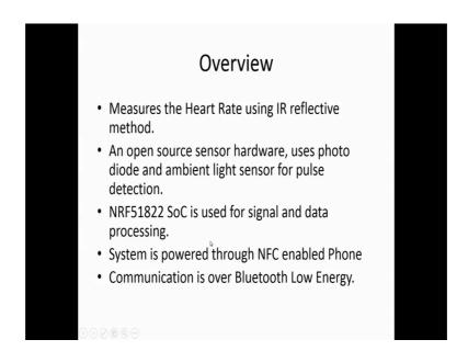
So, what is the overview? It basically measures the heart rate using IR reflective method. It is an open source hardware and it uses a photodiode and ambient light sensor for pulsar detection. I already mentioned to you that we use this NRF 51822 SoC for signal and data processing and system is powered through NFC enabled phone and the communication is true that route B which is essentially the Bluetooth low energy system.
