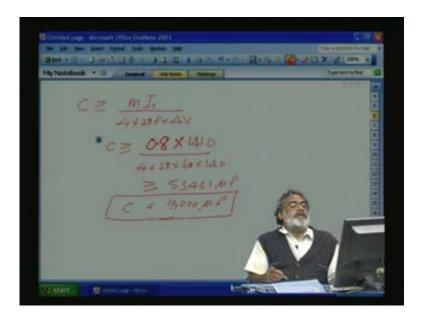
So, this can be further simplified as C greater than or equal to modulation index m into  $I_S$  that I is the input current,  $I_S$  into 4 into 2 phi f into delta V. So, from our data's given, C should be greater than or equal to 0.8 into 1410 divide by 4 into 2 phi into f is equal to 60 hertz into delta V is 140. So, this will give greater than or equal to 5343.1 micro Fahrenheit.
