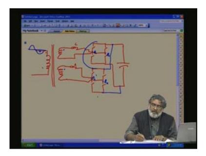
So, you have single phase mains here, the configuration will be like this; this is the transformer, this is our main, single phase. Then we will have the one secondary here, another secondary here. Then you have the inductance here that is L, L here. Then you have one converter here. Here to suppress the next harmonics, second, harmonics at the sidebands of second  $f_c$ , we will use one more converter in series and parallel configuration.
