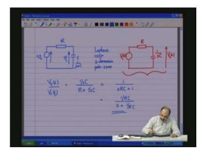
Still further simplifying we can write it as: 1 by RC divided by s plus 1 by RC. So this is the transfer function for this network, for this RC network. What does this mean or what does this imply?
