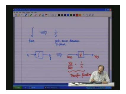
Transfer function is defined as transfer function is defined as the Laplace transform of the output variable by the Laplace transform of the input variable under zero initial conditions under zero initial conditions. This is how a transfer function is defined. And what we got as the transfer function of the integrator which is Y(s) by U(s) is 1 by s under the condition with the integrator initial condition is zero.
