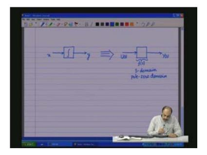
Notice that I have replaced the lower case u by upper case U, lower case y by upper case Y it is just a convention. All the variables in the S-domain or the Laplace domain or the pole-zero domain we represent it with upper case. We now would like to see what is Y(s) by U(s) equal to; this is give the input and output relationship in the S-domain.
