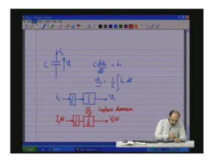
Now let us see that from this we have I c function of (s) 1 by C into 1 by S equals V c which is a function of (s). Or V c by I c (s) function of (s) is given by 1 by sC. Compare this compare with V c by I c functions of time which were equal to 1 by j omega C. This is for the sinusoidal steady-state condition. This we have obtained for the sinusoidal steady-state and this is Laplace domain or the pole-zero domain.
