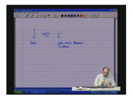
So now the integrator as such with an input u and output y can be represented in the pole-zero domain as..... now the input is a function of s U(s), output is the function of s Y(s) and the integrator can be represented as 1 by s or Y by s the output by the input is 1 by s. In fact, this we call it as a transfer function of the integrator.
