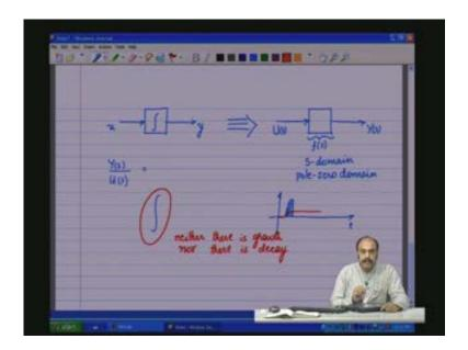
So if we go back to the S-plane let us say I will write the S-plane, you have the sigma and the omega and this is the S-plane and let us say I have a pole there exactly at S equal 0 plus j 0 which means which means at this point if I look at the time evolution which we say is exponential of e to the power of minus 0 plus j 0 into t which is equal to 1 so it is just a constant one, no growth nodes.
