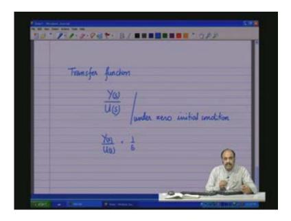
Now we should be able to obtain the transfer function of any circuit and the transfer function of any circuit will be of this general form: Y(s) output variable Laplace transform, input variable Laplace transform equals, it will have a numerator which is a function of a numerator which is a function of s a numerator polynomial a denominator which is a function of s a denominator polynomial.
