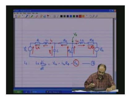
Now these equations 1, 2, 3 can now be put in the standard form of x dot which is equal to Ax plus Bu and y which is equal to Cx plus Du.
