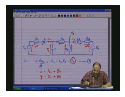
In this case the state vector, x is the state vector which is i L 1 V c i L 2, this is the state vector. There are three state variables, u is the input vector which consists of two V i 1 and V i 2. So you will find i L 1 dot i L 2 dot i L sorry 2 dot..... I made a mistake here I apologise V c dot is equal to the A matrix which is basically the function of all the parameters of the circuit the R 1 R 2 all those things and you have i L 1 V c i L 2 plus the B matrix and V i 1 V i 2.
