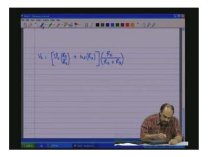
So V x equals V c R 3 by R 2 plus R 3 plus i L 2 R 3 R 2 by R 2 plus R 3. This is the equation for V x which is the intermediate variable that is expressed in terms of state variables.
