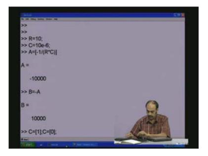
So in this way we can enter and obtain the three matrices which is the A B C D sorry D matrix.
