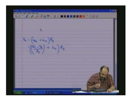
Now let us solve this for V x which will turn out to be V x plus V x R 3 by R 2 equals V c R 3 by R 2 plus i L 2 R 3 and V x is equal to [V c R 3 by R 2 plus i L 2 R 3] this whole thing multiplied by R 2 by R 2 plus R 3 from this equation (Refer Slide Time: 20:37) so from here this can be obtained.
