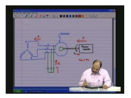
How much is the amount of capacitors that we need to put that would depend upon the amount of flux we need to build up or that is the reactive energy that is needed to build up the flux; probably an example will clarify that particular issue.
