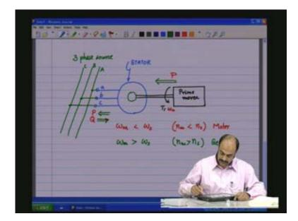
Now, instead of connecting it to a 3 phase source what happens if we connect this to a 3 phase load meaning let us..... so we have and now we have the a, b and c we erase these things okay (Refer Slide Time: 19:05) so now we have a prime mover and this is now connected to let us say a star load. So, instead of a 3 phase source we are connecting the
