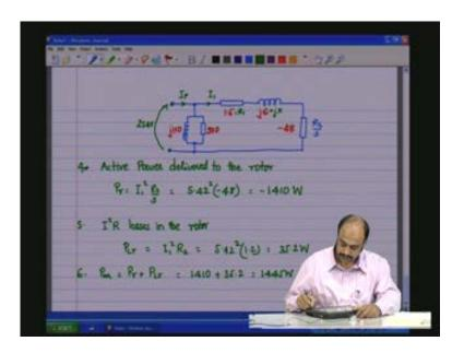
next So the losses in the stator: the I square R losses in the stator is equal to...... P loss stator is equal to I 1 square R 1 which is 5.42 square into 1.5 that is equal to 44.1 watts. The the stator core losses, core losses in stator is given by E square by R m R c which is 900 so 254 square by 900 ohms and that is equal to 71.7 watts.
