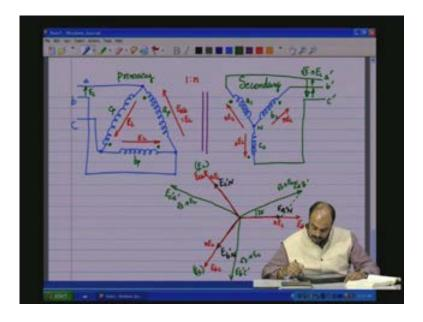
Now you see that the primary three terminals and the secondary three terminals are phase shifted with respect to each other by 30 degrees on top of it the amplitude is root 3 n times if E L is applied what you get at the terminals would be root 3 into n, remember that.
