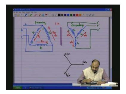
Now the line voltages that is a dash E a dash b dash is 30 degrees leading and I will show that as a different...... this is 30 degrees leading like that the E a dash b dash which is nothing but E a dash N plus minus E b dash N which is what I have shown here and likewise it is 30 degrees leading for oh so E c dash a dash and so on E b dash c dash okay so that is 30 degrees leading.
