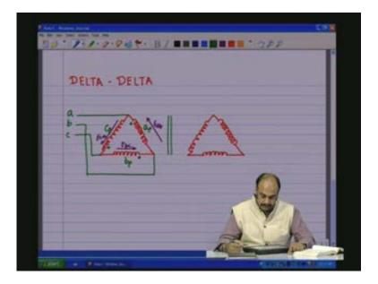
Now, for the secondary for the secondary we have a s coil, the b s coil and the c s coil and let us say the dot polarities are in this fashion as shown so which means the voltage this would be E across coil a s but we will give some point a b a b prime for the secondary or let us say this has a prime attached to that one and this voltage will be E bc prime to indicate it is on the secondary side and we have E ca prime to indicate that it is on the secondary side.
