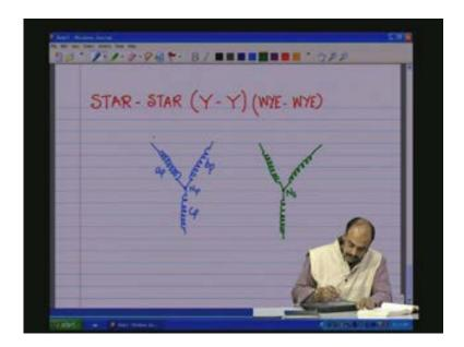
Now, the a phase is connected to the a line, the b phase point is connected to the b line and the c phase is connected to the c line on the primary on the primary. Likewise, on the secondary side you have the a, you have the b and you have the c as shown here. So you have the a prime, b
