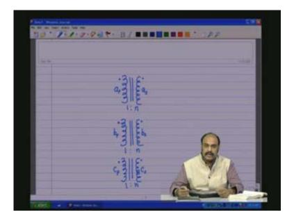
Now the three primary windings can be connected in one of the topology star or delta and the three secondary windings can also be connected in one of the topology that is star and delta which will result in four topologies for the entire transformer.
