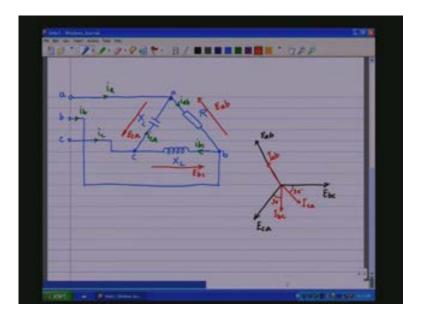
So if I draw extend the E ab line down so you will have a 30 and a 30 here. okay So this is how the phase currents and the line voltages would look like the phasor diagram of such an unbalanced system.
