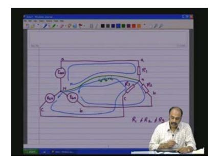
So we have these three independent circuits and the voltages across each phase is E aN, E bN, E cN which is as decided by the source so there will not be any anomalous behavior or any any voltages due to the unbalanced load the voltages across all the 3 phases will still be the same as decided by the load whereas if this green line the neutrals are not connected then the unbalanced currents will flow through will get mixed up and flow through the other loads and then you can
