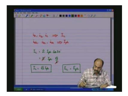
So if we summarize the star and delta circuits so you have the star and you have the delta circuit we can put it like that and this is like this let us say. The star circuit E line equals root 3 E phase I line is equal to I phase and the delta circuit E line equals E phase line voltage is same as the phase voltage and I line will be root 3 times I phase. These are the two important relationships with respect to the star and delta circuits.
