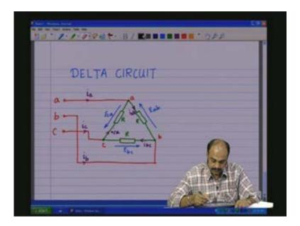
So first let us draw the phasor diagram. So in the phasor diagram we first draw the phasor diagram of E ab E bc E ca. We know that the line voltages are all having the same amplitude same effective amplitudes phasors but they are all displaced 120 degrees out of phase with each
