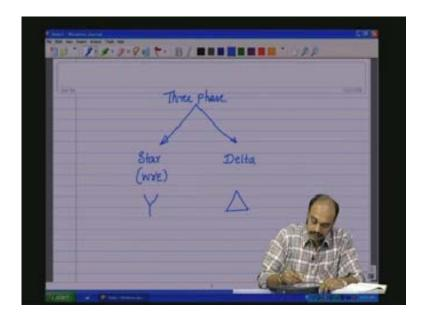
In the in the star circuit we saw that if there is any load one end of the load or the source gets joined connected as shown here and this point is called the neutral point (Refer Slide Time: 3;22) and the other end will of course go to the source. Now these loads we are showing right now as resistive loads but they can also be reactive impedance loads which are the combination of resistance and reactants.
