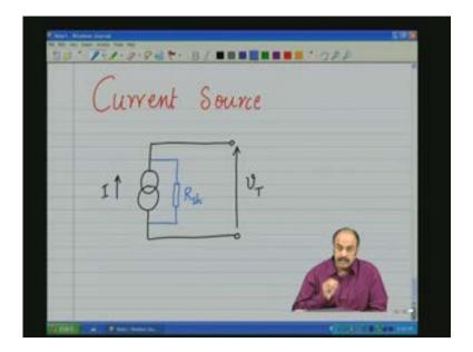
In an ideal source R shunt will be infinite, will be very very high. In the case of a practical current source R shunt is not infinite but a value which is finite but may be in mega ohms and such in that order.
