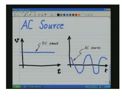
So an AC source the voltage waveform or the current waveform of that particular source varies those positive and negative or has a varying component as a function of time. Whereas in the case of the DC source as a function of time the value of the voltage of the current is going to be constant.
