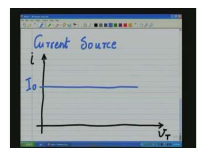
These are ideal characteristics. Only in the ideal characteristic you see the voltage source and the current source I-V characteristic where the waveform is horizontal straight line. But in a practical characteristic it is going to deviate from this horizontal straight line significantly and later on we will see how these non-idealities are going to affect the I-V characteristics of these sources.
