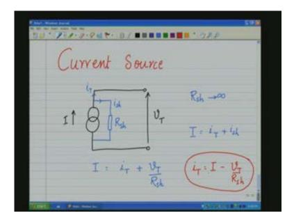
However, in a practical case R shunt is not infinite there is some contribution of this as V T increases from zero to a higher value.
