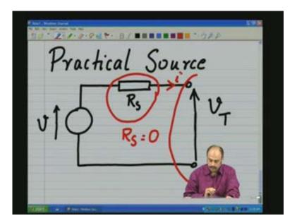
Therefore, now let us have a look at the V-I characteristic of some practical sources. Let me draw a small scale down circuit of a source here (Refer Slide Time: 22:28). Let us construct the source which is comprising of an ideal source V with the non-ideality of series resistance R s and there is the terminal voltage resulting due to connection to the external circuit.
