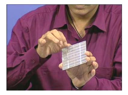
Typically the efficiency of this cell would be around 10 to 12 percent which means if you have 1 kilowatt of energy falling on this terminal power that you would get the electric power that you would get out of this cell would be something like 120 watts. So that is what the order of efficiency would be for any typical photovoltaic cell.
