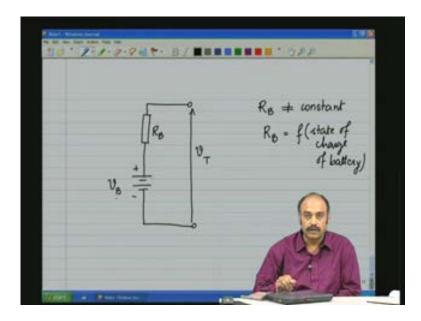
Let us now draw the I-V characteristic of this practical battery that we have been talking about; a battery which is composed of an ideal voltage source DC voltage source in series with the series resistance R B. So the Y axis is the terminal voltage, the X axis is the load current i so this point is load current of 0 amps or open circuit.
