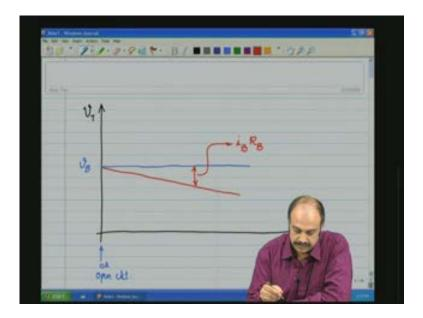
You should know that the battery I-V characteristics that we just saw is more of a general nature. The exact IV characteristic will differ from battery to battery, from the type of the battery to type of the battery, from manufacturer to manufacturer, from ampere rating to ampere rating and so on and so forth. So you should actually take the I-V characteristic data from the manufacturer's data sheet for much more specific details.
