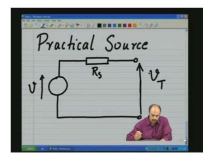
In the case of the ideal source this component was not there; R s was equal to 0 in the case of an ideal source. But in the case of all real practical sources R s is the finite value a non-zero value and it has an effect on the V-I characteristic of the source. So now the V-I characteristic of the source has to be seen with respect to this point (Refer Slide Time: 21:54) so it should be V T versus the current high which is flowing here.
