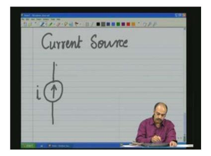
Now this is the terminal and the terminal voltage for the current source is determined by the external circuit. So this is one such representation of a current source. Alternatively you can see a current source being represented in this manner also. A double circle with an arrow indicating the flow of direction of flow of current and an i to indicate that it is a current source and the terminal voltage V T which is determined by the external source.
