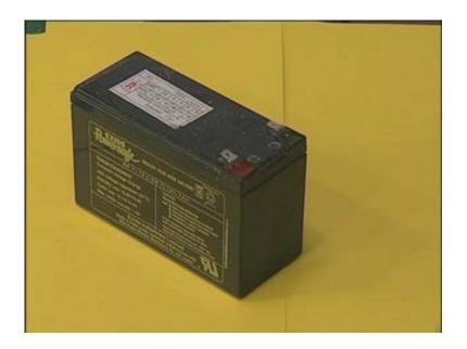
A typical battery looks something like this. There are many types and versions of batteries. This is one such battery. It has two terminals: one marked positive which is red in colour, the other one marked negative. We will have a closer look at the battery shortly. Before that we will try to understand how we represent the battery on paper meaning its symbolic representation.
