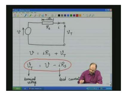
So let us have a look at this equation. Let us picturise it and see how the I-V characteristic looks like. So let me put down that equation here V terminal equals the ideal source voltage minus i into R s. Remember that in the case of ideal source R s is equal to 0 and this component is not there and therefore terminal voltage is same as V. But the practical sources R s is not equal to 0 and therefore this component comes into the picture.
