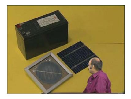
These two sources are DC voltage sources DC voltage and current sources in the case of a solar cell, a DC voltage source in the case of the battery. In the next class we will see the characteristics of the AC source one of the most important sources which is the wall outlet which comes from the wall outlet which is a 230 volt mains.
