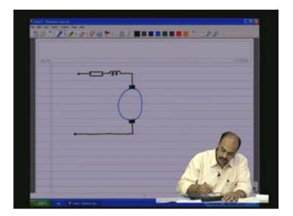
Now this is the DC motor which has a mechanical shaft and we said that in the case of the motor the energy is moving from the electrical domain to the mechanical domain and the mechanical loading gets reflected on the electrical domain as back emf across the brushes.
