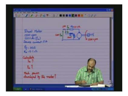
Now let us calculate first I a. now I f is known, easy to calculate which is 120 volts by 120 ohms which is equal to 1 amps. So 1 amps flows through I a, 51 amps is coming from the source so I a is equal to 51 amps minus I f which is equal to 50 amps because I f is 1 amp.
