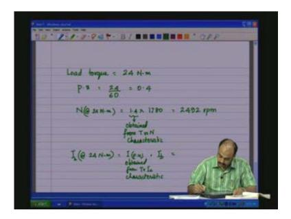
So going back to the characteristic here (Refer Slide Time: 35:35) you will see that the it cuts the torque verses I a curve the torque verses I a curve around 0.6 let us say 0.6 per unit so this will be 0.6 into 54 is equal to around 32.4 amps so this would be the I a and the speed at a torque of (Refer Slide Time: 36:14) 24 Newton meter for a characteristics as given like this for this particular machine. So this how one goes about calculating.
