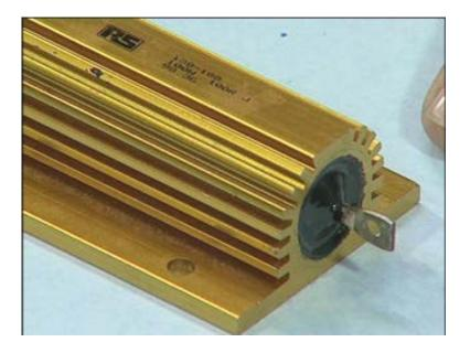
And this has four mounting holes which can be mounted on to another aluminium based plate or base metallic sheet which can dissipate the heat much more effectively.
