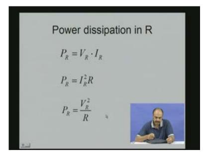
So you see here the summarization of the power. Power is V R into I R, power dissipation in the resistor is also I square R, power dissipation in the resistor is also V square by R depending upon which variables are known at any given point of time.
