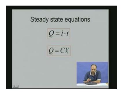
So here are the steady-state equations for the capacitor. The charge Q is related to the current and time in this fashion. The current into time is equal to the charge. The charge is also equivalent to the capacitance or the capacity of the capacitor into the voltage V. Q is equal to CV, Q is equal to i t these are fundamental steady-state relations.
