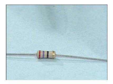
So what you see here is a resistor which has two leads. There is one lead here, there is another lead here which gets connected to your circuit and this portion (Refer Slide Time: 11:38) is the resistive portion which impedes the flow of the current and there is going to be a loss; I square R loss or the V square by R loss or V into I R loss any one of those equations.
