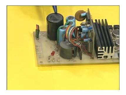
We have the outputs and here is the input, this is followed by a capacitor an aluminium electrolytic capacitor. Here you see three capacitors which are the non-polarised capacitors, there is a board here, it is a piggyback board which is riding on the big motherboard, you see ceramic capacitor here (Refer Slide Time: 59:49) etc so transistor, there is a potentiometer here and whole lot of resistors inside here on the board and you see the power devices mounted on the heat sink here.
