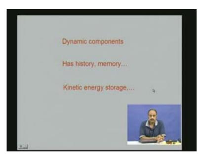
And like in the case of the capacitors the inductors are also dynamic components meaning they can store the state; in this case the flow, the flow would be the current and it can have a memory like the capacitor had voltage as the memory it can have current as memory or the history so it can remember the currents, it can remember the current as a state variable and it stores of course the kinetic energy.
