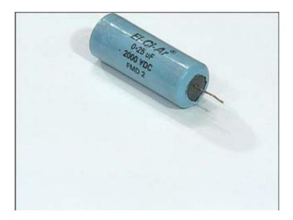
Now here is another non-polarised capacitor which can handle much higher current than the ones you just saw which means that higher current carrying capacitors should have lower equivalent series resistance or ESR. So this is one such non-polarised capacitor normally used for snubber applications. I will also show you another capacitor.
