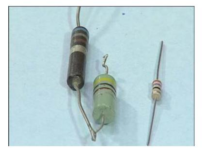
There is this other type of fixed resistor; this is also actually carbon compound. But you see that this is slightly bigger than the half watt and quarter watt resistors to handle much higher power dissipation capability. These are the high wattage resistors which will go in to your circuits. There are still higher wattage resistors available in the market.
