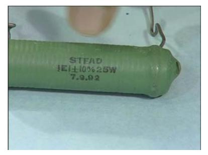
This is a 25 watt resistor, this a wire wound resistor and you will see that the value of the resistors are written on the body of the resistor and here you do not see the colour coding. In fact, in high wattage resistors there are no colour codes but the value is directly written on the body of the resistor.
