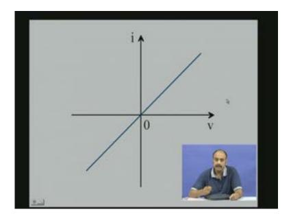
Now coming back to this V-I characteristic let us take a point on the voltage axis and then draw a line directly up on to the resistor characteristic line (Refer Slide Time: 7:40) and from that intersection point we draw another line which intersects the current. So at this point we see that voltage here gets multiplied by the slope 1 by R and results in the current. So you have the voltage multiplied by this resistor resulting in this current.
