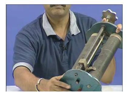
There are two cylinders composed of wire wound wires, this gives the resistors...... they are connected in parallel so that they can handle higher current and therefore more dissipation. This can handle something like 25 amps and they are 2 ohms which means something like 1250 watts.
