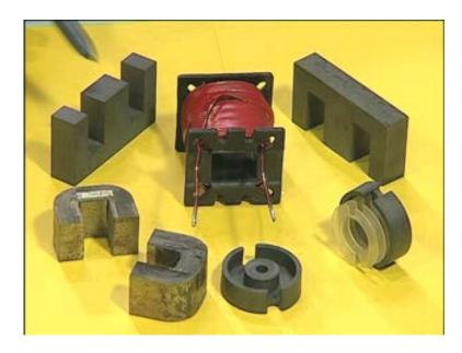
Look at this frame here there are various components. This is an e core one half of the e core. This and this (Refer Slide Time: 55:35) together forms the total core in fact, this will go into this core and this called the Bobbin. On this Bobbin we wind the wires the copper wires; these are copper wires which are wound. And after winding you take this core put it like that and assemble it in this manner.
