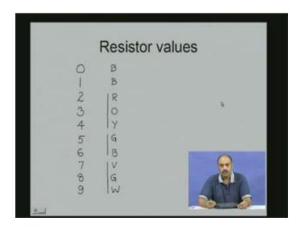
How does one know what is the value of the resistor of a given resistor. Let me show to you a resistor, how practical real world resistor looks like.
