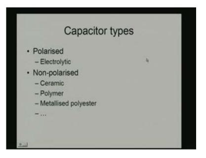
The capacitors also come in various forms, various types and different materials that are used in the manufacture of capacitors. So you have basically two types, broad categories of capacitors: the polarised capacitor and the non-polarised capacitor.
