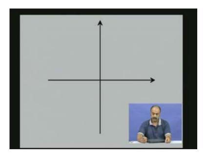
So let us try to characterise these resistors. In fact, most of the components generally we characterized by the iV characteristic. We put the V voltage on the x axis and i on the y axis. So here in this particular diagram V is the independent axis and i is the dependent axis. So in this iV characteristics we plot the character of the resistor as you see here is a straight line and the slope
