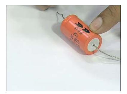
Now this capacitance has leads on this side. This is an axial lead capacitance. It is 4700 Microfarad capacity value. You see the minus sign here with the arrow sign which means this lead is negative which means this lead should be more positive than this at every instant of time so this is a polarised capacitor. Similarly, there is another electrolytic capacitor which I just showed you.
