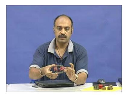
You see here this is a practical real world inductor. You have these two terminals coming out here and there is a core here and the two coils here. Of course here for handling the current rating
