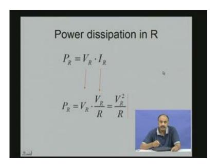
The power dissipation can also be written as V R and I R can be written as V R by R as we saw earlier in the governing equations, this gives V R square by R that is voltage square by R. So, summarizing we see that the power dissipation or resistor can either be I square R if you know the current or if you know the voltage across the resistance then it is V square by R.
