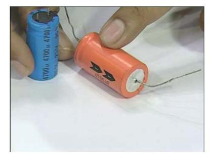
This is radial lead as against the axial lead here. In the market you will find these two types of varieties: the axial lead electrolytic capacitor and the radial lead electrolytic capacitors. The polar polarity is of course indicated here on this type. I will now show you one more capacitor which is still bigger in size.
