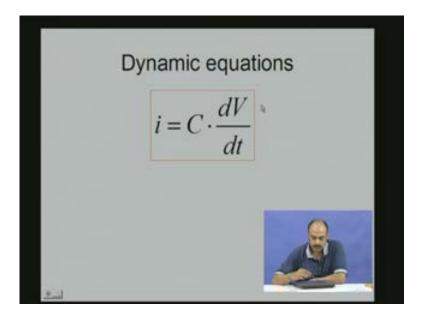
The dynamic equations, the steady-state equation is when everything is under stable operating conditions nothing is varying nothing is changing. In dynamic conditions when there are transients when there are step changes so these are the dynamic equations which are the more general equations; under steady-state constraints you will see the earlier steady-state equations coming into play.
