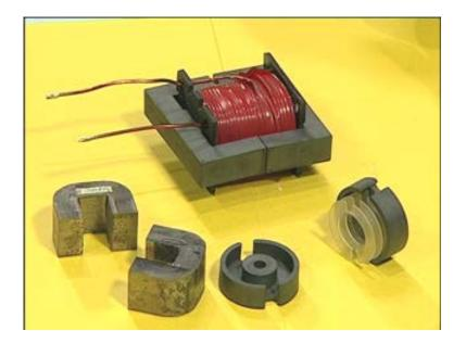
Now this becomes an inductor with a ferrite core. So this is a ferrite core. You have one end of the winding here (Refer Slide Time: 56:16) another end of the winding here goes through this coil there is a Bobbin and this Bobbin is fitted into the core is a ferrite core ferrite EE core.
