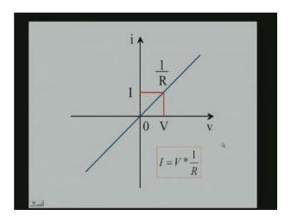
That becomes the governing equation for the resistor I equals voltage V by R or it can also be written as voltage V equals current I into R. It is basically the same equation which is algebraically represented in a slightly different manner.
