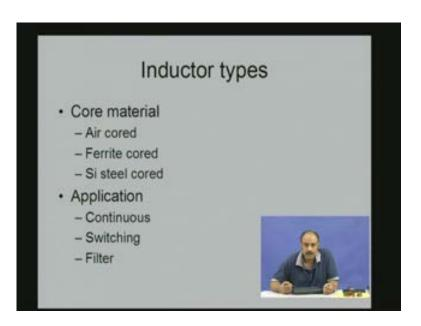
The inductor also comes in different types based on the core materials. We have the air cored inductor, the ferrite cored inductor, the silicon steel cored inductor and also it can be categorised based on applications: the continuous applications, the low frequency applications, the switching applications which are more common, the switch mode power supplies, filter applications which
