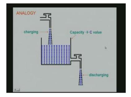
The capacity of this drum or bucket is analogous to the capacitance value of the electrical component capacitor and the height or the head of water that is going to get stored in this bucket is the potential of the energy and that potential is the voltage potential in the case of the
