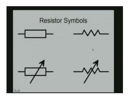
The resistors are shown by various symbols in the textbook. You have a rectangular box with two leads, you have a zigzag set of lines connected to the two leads this is one form of representation and you have a rectangle box and then an arrow in-between to represent a variable
