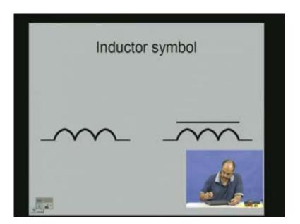
One should note that if one is talking of a saturable core inductor then sometimes in the literature you see a symbol which is like that. Sometimes you will also see a symbol with a double line for the core. These are the various symbols that you will find in the literature but in general the basic symbol is the curved surface the curved lines indicating the coils in an electric circuit.
