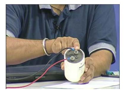
Look at this capacitor. It has two terminals and this is a polarised capacitor. If you can see here there is a plus mark which means that this terminal has to be more positive with respect to this terminal at every given point of time. And here you see the values written; the two main values which we keep looking in the capacitor which is the capacitance value and the voltage withstanding capability (Refer Slide Time: 45:00).
