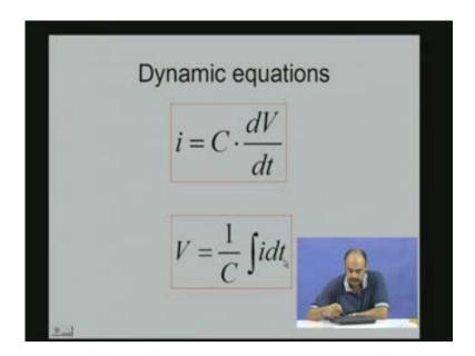
Now this integral here implies that there can be history, there can be initial condition. So the initial condition as far as the capacitance is concerned will be a voltage value. So therefore capacitor remembers voltages, it can remember the immediate past value of the voltages and voltage is the state value or the state variable for the capacitance and in the case the capacitance
