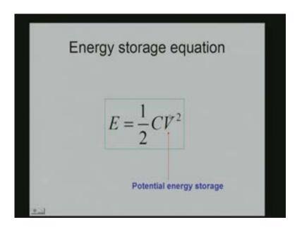
So we say that as the capacitor has the voltage variable here and the energy equation and its state variable of the state value is the voltage or the history that it can remember is the voltage which is the potential therefore it is called the potential energy storage component.
