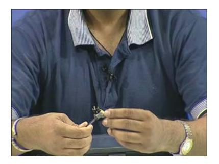
Now here is one such component, this is also a potentiometer similar to low wattage blue box that you saw previously. This also has three terminals. these two (Refer Slide Time: 19:31) are the extreme end terminals of the resistor and this central terminal is the centre tap which actually will vary with respect to the end terminals and the variation of the centre tap can be attained by rotating this vertical knob which is around here.
