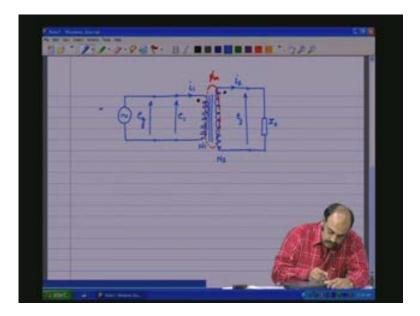
Therefore, for this circuit let us say we have 200 volts 50 hertz as the source and let us say this is 90 turns and this is 2250 turns N 2, let us say that there is a load current of 2 amps that is flowing with a lag angle of with a lag angle theta of cos inverse of 0.8 or power factor equals 0.8. Let us say lagging load which means Z is inductive RL kind of a load.
