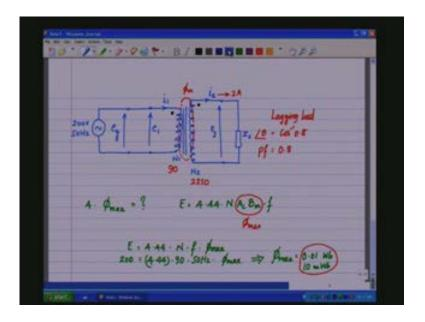
Like this we get the information about the transformer using basically the fundamental laws law which is the Faraday's law of electromagnetism and also one more law which is the Ampere's law. Now let us draw the phasor diagram for this circuit.
