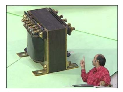
Now you see at the winding at the centre which goes through a central limb. Now this consists of both the primary and the secondary. So the primary is wound first and then the secondary is wound on that one about the central limb. So the core here looks slightly different. Let me give you a better idea by drawing the two dimensional view.
