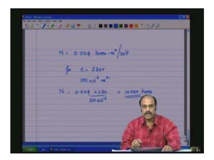
Therefore, a core of this size 100 into 10 to the power of minus 6 metre square core crosssectional area if you want to apply 230 volts you will have to approximately put around 10000 turns so that it can withstand that voltage and deliver the power from the primary to the secondary.
