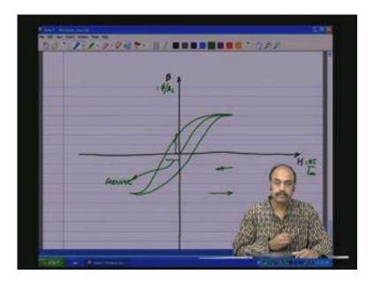
So, a virgin specimen starts with zero and then from there on it exhibits this kind of a hysteresis curve so all magnetic materials will exhibit this kind of a hysteresis curve called the BH loop. So the magnetomotive force which is proportional to the magnetic field intensity is not linearly related to the flux in the core or the flux density d in the core; it is related by this kind of a graph which exhibits hysteresis and this is called the BH curve or the BH loop.
