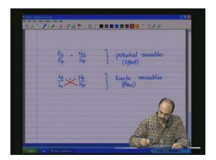
Note here the inverse proportionality e s by e p which is equal to N s by N p; e s is proportional to a proportionality to the turns the number of turns, the current is inversely proportional to the turns i p and N p, i s and N s so that the energy conservation is obeyed so that the power at the primary and the power at the secondary under ideal conditions will be the same.
