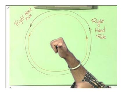
Allow the allow the flux lines, you see the flux lines which are orthogonal in an orthogonal plane to which the current is flowing, the fingers point in the direction which direction in which the flux is going to flow. So as the fingers are pointing here for a current flow in this direction you will see the anti-clockwise direction of the field lines, this is the right hand row.
