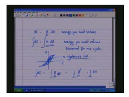
Now the energy including the core volume would be..... so hysteresis energy including core volume is given by half because that was energy per unit volume; this is half BH into V c the core volume. Now the power hysteresis loss is the rate of energy which is divided by the period, one period, so power is 1 by T E h which is half B H V c into f, this is the hysteresis loss equation.
