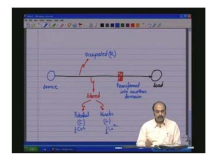
So all these things can happen when the energy emanates from the source and goes towards a sink and load. Three main things can happen which is dissipation in a resistance, storage in a potential form in a capacitance; storage in kinetic form in the inductance and a fourth thing that can happen is yet transform into another domain. These are the things that can happen. This we have discussed earlier.
