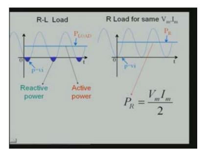
So P load is definitely going to be less than V m I m by 2. So, for a sine waveshape of phase angle let us say phi of current with respect to the voltage, this P load will turn out to be V m I m by 2 cos phi, how is this obtained; this is nothing but integral of V m sin omega t into I m sin omega t minus phi divided over by the period t. So this will result in V m I m by 2 into cos phi.
