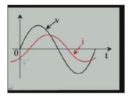
Here notice that the red colour current waveform is lagging the voltage waveform by an angle phi. This is an RL load (Refer Slide Time: 28:28). If the current waveform were in-phase at zero with a with respect to the voltage waveform then it could have been a pure resistive load and if it had been exactly at this 90 degree point then it is a pure L load and if it had been exactly leading by 90 degrees somewhere here it would have been a pure C load.
