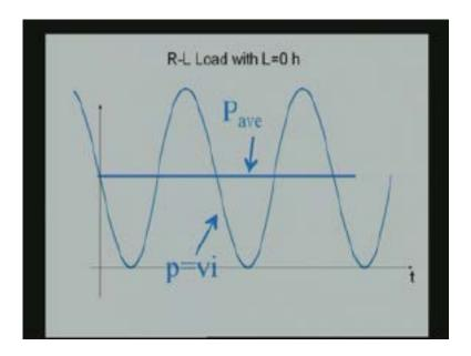
So when R starts increasing towards a very large value you will reach the condition like a pure resistive load or L is equal to 0 Henry load that kind of a situation. So you see the way the power curve transforms as you increase the load and this is as you decrease the resistance.
