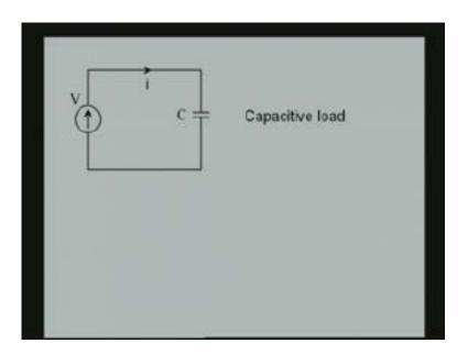
Here the load is a capacitive. Let us apply the same sinusoidal voltage waveshape through this capacitor on this capacitive load and see what happens to the current waveshape under steady state conditions again (Refer Slide Time: 05:15).
