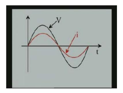
We have here the x axis which is the time axis and y axis the amplitudes, the black curve is the voltage waveshape which is the sinusoidal voltage waveshape, and it is a source voltage. The red colour as you see is the current waveshape. So, for a resistive load pretty simple, you see that the current is in-phase with the voltage because it is just V by R.
