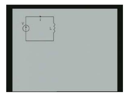
Now consider instead of a resistive circuit an inductive circuit, the load is inductive because the R has been replaced by L here as you see. Now what happens if we apply a sinusoidal voltage to this inductor under steady state conditions?
