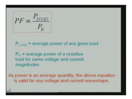
One thing you should keep in mind here is what would happen what would happen if the power factor is low. So the power factor is low it means that P load is low and this P load is low which means that there is a quite a difference between P load and P R for the same I m V m.
