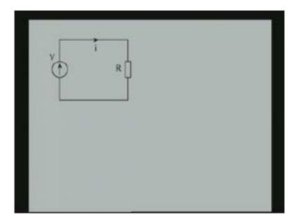
It is a simple circuit with a voltage source of an arbitrary waveshape and also consists of a resistance, it is a resistive load, and as shown in the diagram there is a current i also flowing through it.
