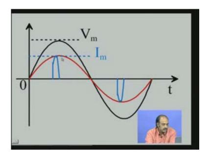
So let us compare V and the red coloured current waveform for a pure resistance, V and the blue coloured current waveform for the capacitive circuit.
