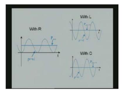
You see that with R you have a power waveform twice the frequency of the input sinusoidal voltage waveform but it is shifted DC shifted as you see and has a finite and therefore as a finite average power non-zero average power. In the case of the inductive load and the capacitive load the average power is absolutely zero; only that the power waveform is having a 180 degree phase shift with respect to each other. So this is the comparison of the power waveform for the R, L and C circuits.
