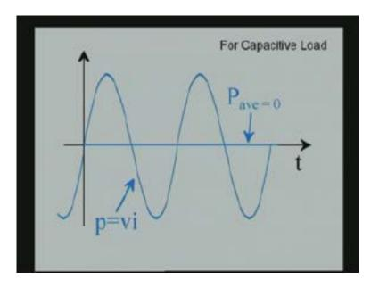
The capacitive circuit also results in an average power equal to zero interesting is it not? Only the resistive circuit gives a finite average, keep that in mind because we will be using it much later. So let us put them altogether and compare.
