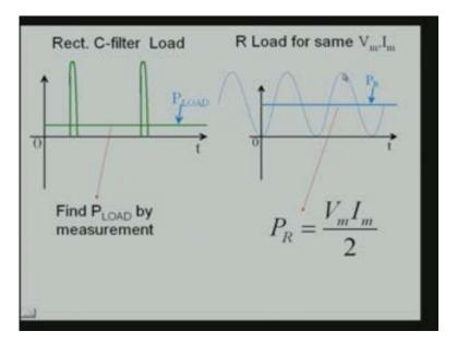
This point here or the cursor point is V m I m and this will be the average value which is V m I m by 2 and this P load the average will of course will depend upon the actual load it will actually depend upon the area under these curves for which we can get the measurement which I will tell later on.
