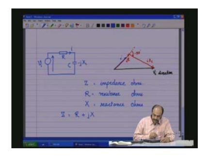
When you look at this phasor diagram here it could be either the v i direction phasor diagram or the i reference phasor diagram, this is i into R, this phasor is i X c, (Refer Slide Time: 17:57) this phasor which completes the Kirchhoff's voltage law is i into Z. therefore, let me choose that.
