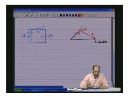
Just to recap, note one point. This j here (Refer Slide Time: 9:16) can be treated as an operator called j operator. Whenever you have multiplication by j into something then this quantity is going to be phase shifted by 90 degrees anti-clockwise. Internationally there is a convention for signs of rotation; anti-clockwise is positive direction for rotation and clockwise is negative direction for rotation.
