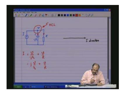
So we have....... so let me put it like this; we have a voltage v direction. So in that v direction there is one vector which is along it and I will call that one as v by R. Now v by R plus j v by X c..... now v by X c is multiplied by j which is along this it is plus 90 degrees so anti-clock anti-clockwise direction 90 degrees which will be like that this is v by X c (Refer Slide Time: 28:17) that is going to give you I is it not.
