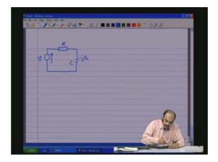
Now let us take a reference which is the v reference or the voltage reference. Now there is a current which is flowing through the circuit and that is i. Now this being a capacitive circuit this current i has to lead the voltage.
