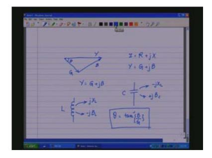
So you see that if we use KVL for solving a loop equation we would land up with an impedance triangle. If we use KCL to solve a nodal equation node voltage equation then we would land up with an admittance triangle. There is one more triangle which you will come across and that is the power triangle. Let us see what this power triangle is.
