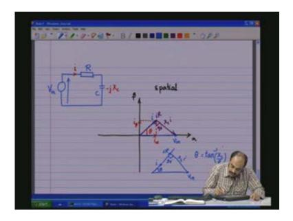
Therefore, knowing the value of C here knowing the value of omega knowing the value of R here you can estimate the phase angle theta which this vector is going to be displaced. Therefore I know that the current is going to lag lead the voltage by this angle theta as decided by the frequency, the capacitance value and the resistance value. So that is the important of this space vector concept.
