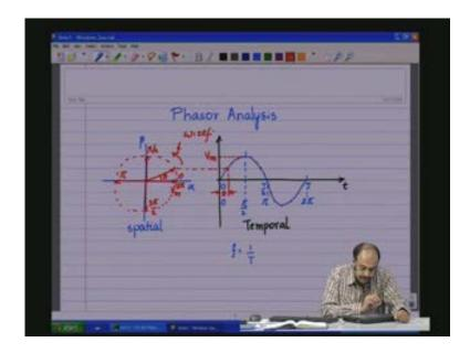
So now that we have an idea that a sinusoidal waveshape can be represented in this spatial coordinates by a single vector, at any given point of time the vector is in that special coordinates anchored at the centre at any position or angle corresponding to the time which is 0 to 2pi in the case of the spatial coordinate system.
