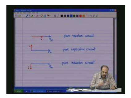
However, in actual practice and real circuits we will not see pure resistive or pure capacitive or pure inductive circuits; it will generally be a mix up piece so we do not get the current leading or lagging by exactly 90 degrees so it will be somewhere in-between depending upon the values of the resistance, the values of the capacitance, values of the inductance and so on.
