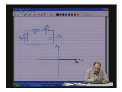
Now let us say for example the capacitance dominates which means the current is going to lead. So now to apply the Kirchhoff's voltage law how do the currents look like; how do the voltage using this current how will the voltages across look like?
