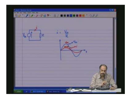
Now if I project this into the spatial coordinates the alpha beta coordinates let me start by taking V in as my reference. So V in is something a vector with an amplitude V m then another vector we will call that one as i vector which is having an amplitude V m by R and that is also in-phase because both are starting from zero that is also in-phase with some value and that would be the i vector.
