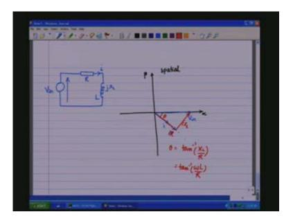
Here also you see that the voltage across R V R, the voltage across L V L vectorially add up to equal V in they vectorially add up to equal V in, such that the voltage across the loop is zero, Kirchhoff's voltage law is valid and thereby upholding the principle of energy conservation.
