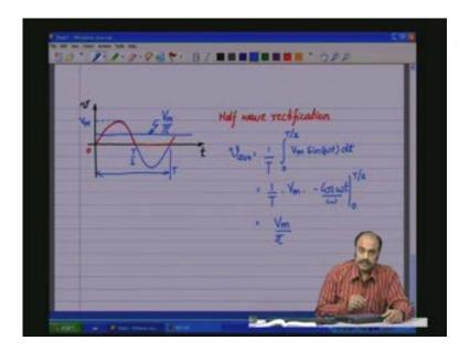
So this is how you obtain the average. There is one more important feature which is commonly used everywhere that is the Root Mean Square or the RMS value RMS value of the sinusoid. What does RMS value mean? This has a relation to the power. It is that value of the voltage or that value of the current which relates to the power or which is the power generating or the power producing part. Therefore let us first look at how the power waveform looks like.
