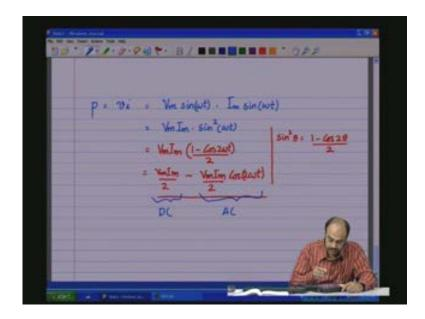
Now if you draw only the power curve versus time, power which is equal to V into i so there is a DC term. So let me write it in dotted blue dotted here, this is the DC term which is V m I m by 2 and there is a varying term or the AC term which is which starts from zero, you have a kind of a waveform which is like that sinusoidal in nature about the DC term and so on its keeps going. So if you take this point to this point that would be T the zero this is T. So this point would be T by
