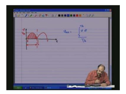
So we know what V is, therefore V average which is equal to 2 by T integral 0 to T by 2 V m sin (omegat) dt which is equal to 2V m by T; integral of sin omega T is minus cos (omegat) by omega by omega and that has to be evaluated at T by 2 and 0 which will give you 2V m by omega T and minus...... now this will be minus cos (2pi by T into T by 2) minus of minus plus so cos 2pi by T into 0 so this is going to be 2V m by omega T into cos of...... so if see
