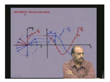
Lecture 9 brings you the concepts of the phasor, the vector, the space-vector, space-phasor because in the analysis of the electrical circuits and especially when sinusoids are used the phasor diagram are used extensively to analyse or represent the circuits pictorially and therefore it is important to understand the concept of the phasor notation and what it means by a space phasor.
