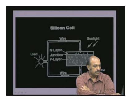
Schematically you will see the lot of free electrons get generated which go into the conduction band because it absorbs the energy from the sunlight and they flow in the external wire to supply the various loads.
