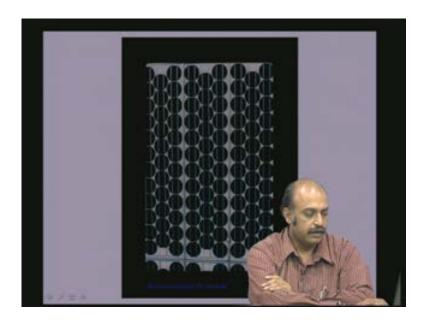
This is also a photovoltaic panel; these are monocrystalline photovoltaic modules available in the market. These modules are available in the wattages of around 36 watt modules or 44 watt modules that are pretty costly today. Of course the costs are coming down. It averages somewhere around 180 rupees per watt.
