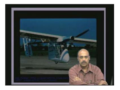
Another application here you will see this is the solar challenger which is run purely by solar photovoltaic cells. We will see the photovoltaic cells are on top here on the wings. It contains something like 160000 cells at 2.7 kilowatt rating.
