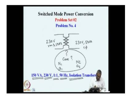
Let us see an example where we want to design a transformer whose V A rating is 150, that is rms voltage multiplied by rms current is 150 and it is a 1 is to 1 transformer. That is primary voltage and secondary voltage are equal. Such transformers are used mainly as isolation transformers the purpose is to electrically isolate, but not modify the frequency or voltage.
