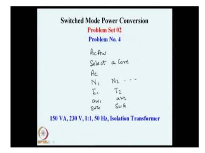
Now, the design of the transformer followed the similar kind of procedures that we had seen earlier then we were explaining about the transformer, that find out the core product, select a core, then for that core find out A c. Find out the number of turns N 1 N 2 etcetera and then find out the currents I 1 I 2 etcetera.
