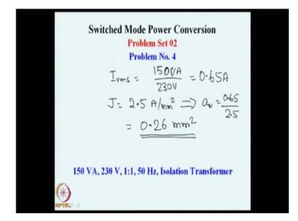
We might go to the next step and see, what is the rms current is 150 V A divided by 230 volts and that number is 0.65 amperes. So, with the current density of 2.5 ampere per millimeter square, this leads to wire cross section of 0.65 divided by 2.5 that is 0.26 millimeter square. So how do we select this cross section of the wire? We again go back to the table that we had here. So, if I open this wire data here which is given.
