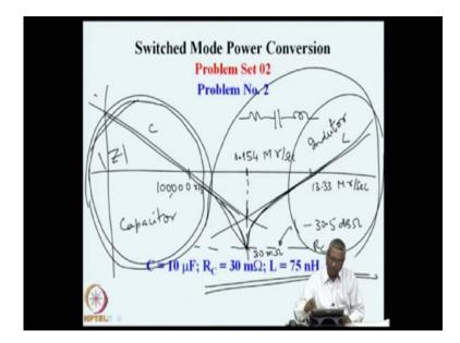
So, if we put all three and try to find out the overall behavior R C L C this is 100,000 radian per second, this is 13.33 mega radian per second and this is the 30 milliohm or minus 30.5 d B ohm and because this is a series circuit R C and L at any frequency. Whichever component is the highest value will dominate.
