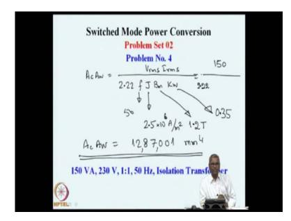
In this particular example, we might go through this process and see that A c A w is the product which is V rms I rms and that product is 150 V A which is given to us, divided by 2.22 f J B m and K w.
