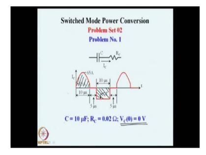
In the same problem if we go, we might also like to find out what is the voltage across the capacitor under the steady state condition. We know that during the positive charging capacitor voltage will build up and during the negative charging capacitor voltage will decay. We start with an initial voltage of zero volts so it is possible to find out how this voltage will.
