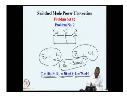
We will move on to understand the capacitive circuit elements in a little more detail. What we see here is a capacitor whose value is as before, 10 microfarad and this capacitor also has a parasitic inductance of 75 nano henry and parasitic resistance of 30 milliohm and in a circuit schematic it is shown as the capacitor that is desired and the parasitic value of inductance which is part of this capacitor and the parasitic value of resistor which is part of this capacitor.
