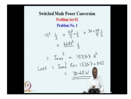
So, now we can put all these things together to have a first term which is 15 square into 1 by 3 plus second term is 50 square by 2 into 1 by 3 plus a third term is 30 into 100 by pie into 1 by 3 plus the portion corresponding to this which is 46.83 square into 1 by 3 so, this is I rms square so, this turns out to be 1533.7 ampere square so, the loss is I rms square into R C which is 1533.7 multiplied by 0.02 which is 30.67 watts.
