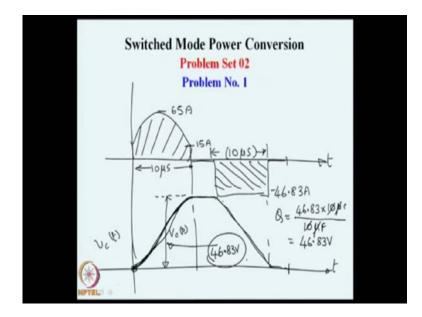
For example, if we see the current waveform so, if we draw these we can see that initially the voltage across the capacitor is 0. So, during this time the capacitor will charge up because we are applying coulomb into the capacitor so it would charge up following a waveform which is integral of this.
