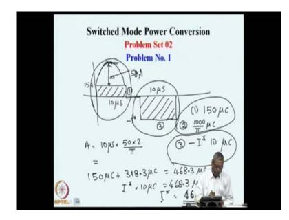
So, there is one section of current which is 15 amperes and 10 micro second. So, this area is 150 micro coulomb, 15 into 10 micro second into ampere is micro coulomb. So, this is the first area. Then, we have a negative area which is minus I star and for again 10 micro second. So, this area can be written as minus I star into 10 microcoulomb.
