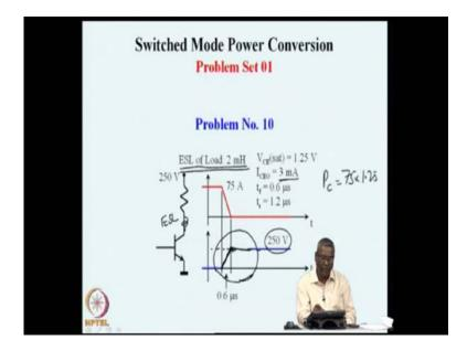
Another issue that we would like to see is, this resistance is not a pure resistance but, it has an equivalent series inductance of 2 millihenry. What is the consequence of that on
