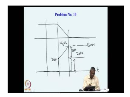
So, just before turning of just before completely turning of, the voltage goes to the peak of 500 volts which is the resistor drop plus the inductive drop. The supply voltage plus the inductive drop and that is what we had seen in this particular example.
