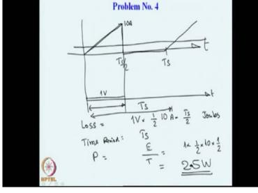
there are no losses and so, we can say the total period for which this loss is taking place is T s. So, the average power loss is energy loss divided by time and that would be 1 into 1 by 2 into 10 into 1 by 2 and that is 2.5 watts.
