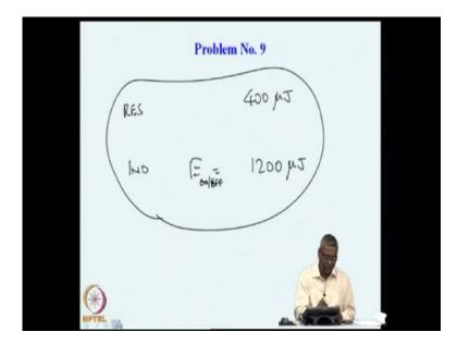
And so, we can say that the total power loss is 1200 microjoule on to off. This is inductive. And if the same thing was resistive, we saw that this was only 400 microjoule. That was a previous example that we had seen.
