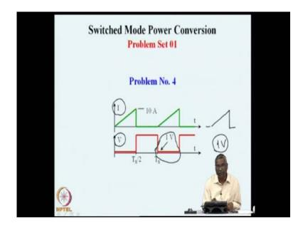
Let us now go to the next problem which is more to do with the losses in the device, the current that is carried, what kind of losses happens while it is conducting and so on. So, what is shown here in this slide is what you see here in this slide is the current through a particular switch and the voltage across the switch in a circuit. When the switch is on, the
