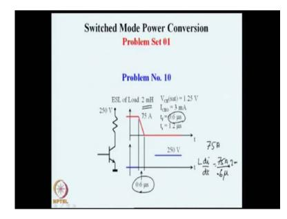
The duration is, this duration is 0.6 microsecond and the current that is dropping is 75 amperes. So, you can see that during this time there is a d i by d t experience and the L is 2 millihenry. So, we can say that during that time this L d i by d t is 75 ampere is d i, time is 0.6 micro 0.6 micro and then, L is 2 milli.
