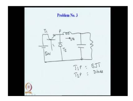
So, you see that the circuit switch has T 1 P is realized by a BJT T 1 P is realized by a BJT transistor and T 2 P is realized by a diode. So, that is how you try to select in any application the switches that are used by electronic devices.
