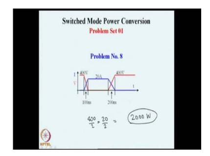
So, the important point to be seen is that when the voltage is falling linearly and the current is also falling linearly, the power dissipation peak power dissipation occurs somewhere in the middle of this and that peak power is 400 by 2 multiplied by 20 by 2 is 400 into 20 divided by 4 that is, roughly 2000 watts. This is the peak power dissipation. Both during on time and off time, the peak power dissipation occurs exactly in the middle and that is 2 kilo watt.
