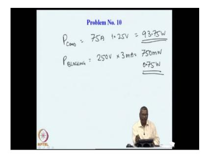
Or if we go, we can say that P conduction is 75 amperes into 1.25 volts and this number is 75 into 1.25 is 93.75 watts. So, let us see what is the blocking loss? Blocking loss is when the device is off there is a leakage current of 3 milliamperes, what you see here; leakage current of 3 milliamperes and the device is blocking 250 volts. So, we can say that blocking loss is 250 volt into 3 milliamperes which is 750 milliwatt or 0.75 watts.
