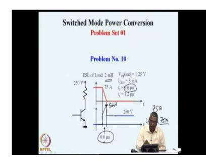
So, what we notice is that, in this example the voltage jumps off to that nature, additional voltage of 500 volts at this point.
