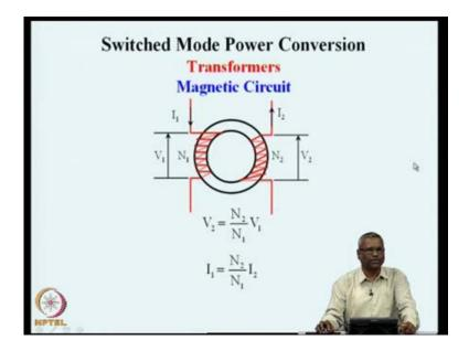
Physically a transformer has a magnetic circuit and electrical circuit. The electrical circuit in this particular situation consists of two parts, a primary the red winding shown here and the secondary winding shown in red color here and the same schematic I have now shown physically through a toroidal core. The shape is not very important we will see later. There are many preferred shapes are available we will see from the standard data sheets the different kinds of core shapes are available.
