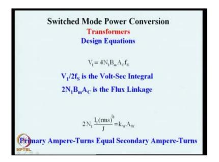
Now, if we combine these equations design equations, where the total number of turns multiplied by the cross-section area of each of the turns is related to the window area and the voltage of excitation is related to the core area and frequency, if these two equations are combined together,
