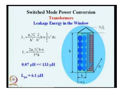
We find that for this particular example the leakage inductance is 0.07 micro Henry and this has to be compared with magnetizing inductance which is 133 micro Henry, the
