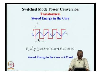
The stored energy in an ideal inductor ideal transformer was 0, but because of this magnetizing current there is a finite stored energy one half of 1 m I m square and that is 0.22 milli Joule. This is another non-ideality ideally this should of been 0, but in real transformer the stored energy is a finite quantity, but it is a small quantity.
