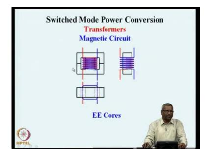
Now, the kind of the cores that we had used for inductors, EE cores are also suited for transformers. In this circuit instead of a ring core, I have e shape core 2 2 pieces of e shapes, they are put against each other so that you have a close to magnetic circuit and in the central limb both the primary winding the red color winding and the secondary
