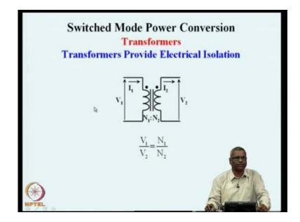
The transformers are also used for providing electrical isolation between one part of the circuit another part of the circuit as I had said, the primary excitation sets up in the core a
