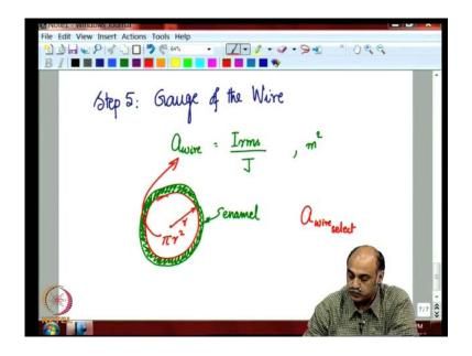
Then, step five, now step five, you need to find out the gauge of the wire, the cooper wire. You recall that in the last class, we discussed about a wire, the cross section of the wire which is equal to Irms, current flowing through the wire and the permissible current density in ampere per meter square. So, you have the rms current in amps by the current density amps per meter square how much you want to permit and you get the wire cross section square wire cross section area in meter square.
