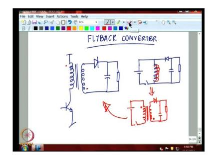
Now, let us just see one more, the fly back and then conclude. The process is exactly the same. Only the fly back convertor as you know, is nothing but exactly like the non isolated buck used, but you have a winding, another winding across which it is connected. So, how you go about this convertor, sorry for this convertor? Now, you see this similarity. If you are using a non isolated buck boost, you would have done it like this.
