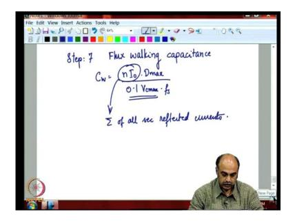
Then, you need to rate the flux walking capacitance, step seven, flux walking capacitance, which is the primary capacitance the one in series with the winding to prevent saturation, flux walking saturation that may happen due to the non idealities and non matching power semi conductor devices. So, the flux walking capacitor can be the designed by allowing some 10 percent drop across it and this.
