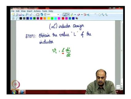
So, let us consolidate the inductor design. So, step one, obtain the value of the inductor. Obtain the value L of the inductor. This is normally obtained using the Faraday's law, the Faraday's equation v L is equal to L d i L by d t. You try to obtain this knowing all other aspects of the faraday's equation. So, this is step one. So, let me name that as step one.
