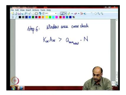
Then, step six, so in step six, you make the window area cross check. So, what is said that we need to check? We need to check that Kw Aw, window factor into the window area is greater than the a wire selected, the selected wire cross section area into the number of turns as calculated in step four from the permeance value. So, if this inequality is satisfied, then you go to the step of actually winding them. Then, you have your inductor which can be inserted into the DC DC converter circuit.
