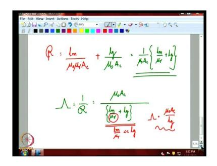
The reluctance is reluctance is lm by mu naught mu r Ac plus the air gap portion mu naught Ac because the relative permeability for air gap is 1. So, this is the reluctance. We can we can take out mu naught Ac. You have lm by mu or plus lg. So, this is the reluctance. What is the permeance? Permeance is nothing but 1 by reluctance. That is given by mu naught Ac by lm by mu or plus lg.
