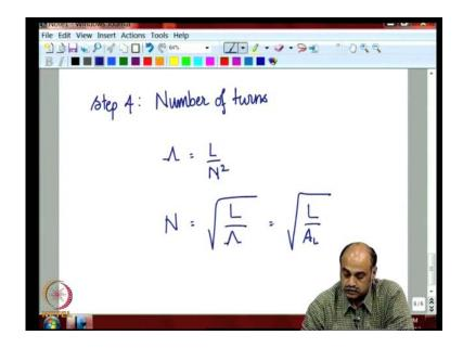
Therefore, we come to step four, which is calculation of the number of turns. The permeance is nothing but L by N square. N is nothing but root of L by permeance. If the AL factor that is given into the root of L by AL and this way, you calculate. This way, you calculate the number of turns.
