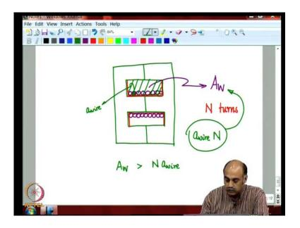
If you see, we have this core. Let we take simple ee core which is like this. So, this is ee core. You have 2 ee core joined together. The former comes in here. The red line indicates the former. The red line indicates the former. Also, this is, on the former is wound the windings. So, you will see windings wound in this fashion. You will see the other end of the windings also here.
